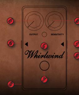
INPUT JACK Connect a cord from your instrument here. Removing the cord from the INPUT jack when not in use disconnects the battery which will prolong battery life.
