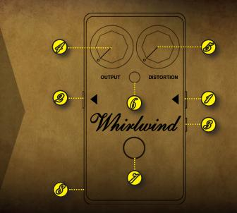
1: INPUT JACK Connect a cord from your instrument here. Removing the cord from the INPUT jack when not in use disconnects the battery which will prolong battery life.
