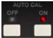
After Auto Calibration occurs, the automatically adjusted parameters can be modified to any other value if desired. If a calibration parameter is adjusted while Auto Cal is ON, the ON LED illuminates in red instead of green, indicating that the system is no longer in the calibrated state. If the moved controls are subsequently returned to their original position, the LED will return to its green state, indicating the unit is back in calibration.
