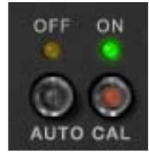
When Auto Cal (Automatic Calibration) is ON in the plug-in, these calibration controls (see [Figure 135 on page 435](#)) are automatically adjusted to the calibrated values whenever the Tape Type, Tape Speed, and Emphasis EQ are modified. After Auto Calibration occurs, the automatically adjusted parameters can then be modified to any value if desired.
