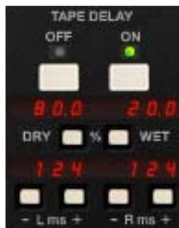
These parameters control the built-in Tape Delay, which creates tape echo effects. For an overview of this feature, see [“Tape Delay”](#) on page 22. The Tape Delay controls are not available in the original hardware.
