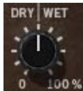
When the plug-in is used in Reverb mode in a track insert (versus effect send/return) configuration, Dry/Wet determines the balance between the original dry signal and the processed signal. The range is from 0% (dry, unprocessed) to 100% (wet, processed signal only).
