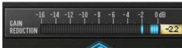
The Gain Reduction meter displays the amount of gain reduction occurring within the compressor.
