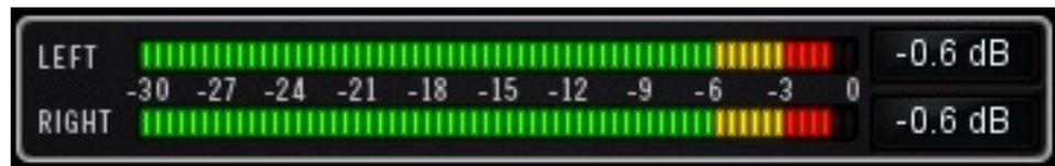
The stereo peak/hold meters display the signal level at the output of the plug-in. The meter range is from  $-30$  dB to 0 dBFS. Signal peaks are held for 3 seconds before resetting.
