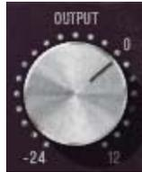
The Output knob controls the signal level that is output from the plug-in. The default value is 0 dB. The available range is -24 dB to 12 dB.
