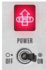
This toggle switch enables or disables EMT 140. You can use it to compare the processed settings to the original signal, or to bypass the plug-in which reduces (but not eliminates) the UAD DSP load (unless *UAD-2 DSP LoadLock* is enabled). The red EMT power indicator glows brighter when the plug-in is enabled.
