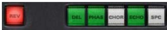
Click a Mode button to activate that program mode; the button is illuminated for the currently active mode (only one mode can be active at a time). Each program mode and its associated parameters are described in detail below.
