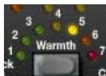
This button defines the Warmth amount. Warmth simulates the softening of the high frequencies that occurs with analog tape saturation (see “Warmth Processor” on page 102 for detailed Warmth description). Higher values increase the Warmth, as indicated by the Warmth Meter.
