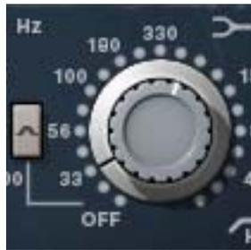
The low band delivers smooth low frequency shelving or peak equalization. The inner knob controls the band gain, and the outer ring selects the frequency or band disable.
