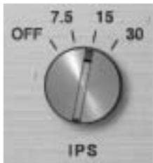
The IPS (Inches Per Second) control determines the speed of the tape transport and the associated “head bump.”
