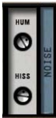
The Noise controls allow the user to control the Hum and Hiss elements found on the original hardware. Separate controls for Hum and Hiss are available and each can be adjusted for creative purposes.
