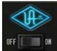
The Power switch determines whether the plug-in is active. This is useful for comparing the processed settings to the original signal or bypassing the plug-in to reduce the UAD DSP load (load is not reduced if *UAD-2 DSP LoadLock* is enabled).
