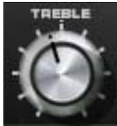
This knob controls the high frequency response in the tape echo portion of the signal. It does not affect the dry signal or the reverb signal. This is a cut/boost control; it has no effect when in the 12 o'clock (straight up) position.
