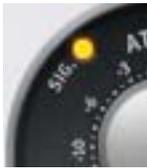
This 4-stage “LED” indicates the presence of audio signals at the input of the plug-in. When the input signal is below  $-25$  dB, the indicator is off. At  $-25$  dB to  $-19$  dB, the indicator glows slightly. At  $-18$  dB to  $-10$  dB, it lights with medium intensity. At  $-9$  dB to  $0$  dB, it shines brightly.
