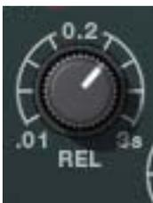
Release sets the amount of time it takes for processing to engage once the input signal drops below the threshold level. The available range is  $10$  milliseconds to  $3$  seconds.
