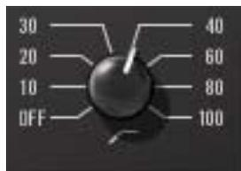
The high-pass filter is useful for reducing low frequency content. It is a global filter; it always affects both left and right channels, regardless of the active mode. See [Table 27](#) below for available settings.
