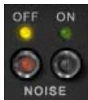
The Noise Enable buttons are a global enable/disable control for the individual hum and hiss components of the A800 model. The amount of hum and hiss noises are continuously variable and are set with the [Hum Noise](#) and [Hiss Noise](#) controls ([page 436](#)). Click the Noise buttons to alternate between OFF and ON.
