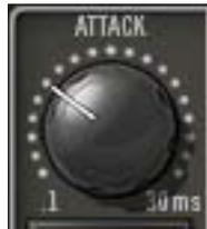
Attack sets the amount of time that must elapse once the input signal reaches the Threshold level before compression is applied. The faster the Attack, the more rapidly compression is applied to signals above the threshold.
