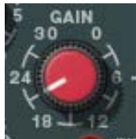
The Gain control adjusts the output level of the limiter/compressor module. The available range is 0 dB to 30 dB.
