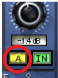
The A/B Selector switches between two separate sets of Cambridge EQ plug-in values. This feature enables easy switching between two completely independent EQ curves which can be useful for comparison purposes or for automating radical timbre changes. Both the A and B curves reside within a single Cambridge EQ preset.
