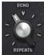
This knob controls the repeat level (feedback) of the echo signal. At the minimum (fully counter-clockwise) position, only one repeat is heard. Rotating the control clockwise increases the number of echoes. Higher values will cause self-oscillation.
