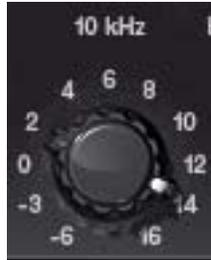
The High Shelf Gain knob offers fixed frequency shelving equalization at 10 kHz. This stepped control can cut the treble by -3 dB or -6 dB, or boost it in 2 dB increments up to +16 dB.
