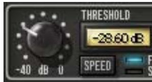
Threshold controls the amount of de-essing by defining the signal level at which the processor is activated. Rotate Threshold counter-clockwise for more de-essing.
