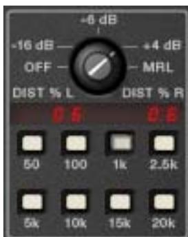
These controls are the suite of tools included to perform manual calibration of the recorder. These UAD-only tools are not in the original hardware. Manual calibration is entirely optional, as the [Auto Cal](#) feature can quickly and automatically calibrate the system.
