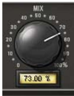
The Mix knob is a mix control for the plug-in. Mix determines the balance between the original and the processed signal.
