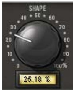
The Shape knob is the primary saturation control for the Maximizer effect. It contours the harmonic content and apparent dynamic range of the processor by changing the small-signal gain of the saturator. The available range is 0–100%.
