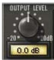
Output controls the signal level that is output from the plug-in. The default value is 0 dB. The available range is  $\pm 20$  dB.
