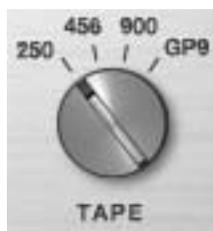
Tape Type selects the active tape stock formulation. Four of the most popular 2" magnetic tape formulas are modeled in the A800 plug-in: 250, 456, 900, and GP9. Each type has its own subtle sonic variation, distortion onset, and "tape compression" characteristics.
