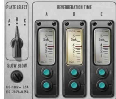
The original damper controls are remote control devices, usually found somewhere near the control room for quick access. Our hybrid panel combines three remotes into the panel, with a switch to select each of the three available systems.
