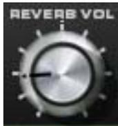
This control determines the volume of the spring reverb effect. Rotate the control clockwise for more reverb. Reducing the control to its minimum value will disable the reverb.
