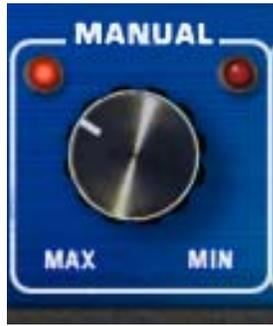
This continuous control determines the delay time of the processor. The delay time is modulated by the Sweep LFO when the Width value is higher than 0%.
