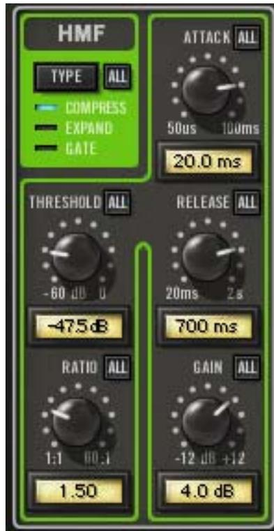
The Band Controls contain the parameters that are used to specify all the settings for each band (except the frequencies; see “Frequency Controls” on page 352).
