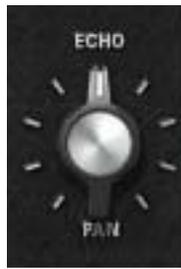
Pan sets the position of the delayed (wet) signal in the stereo field; it does not affect the unprocessed (dry) signal.
