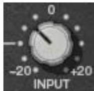
Input controls the signal level at the input to the plug-in. The default value is 0 dB. The available range is  $\pm 20$  dB. Increasing the input may result in more compression, depending on the values of the Threshold and Ratio parameters.
