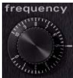
This control adjusts the target frequency of the effect. Frequencies above the current setting are boosted by the amount set with the Amplitude control. Frequencies below the current setting are attenuated by  $-24$  dB per octave.
