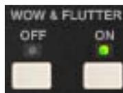
These buttons are global enable/disable controls for the Wow and Flutter effects. When Wow & Flutter is ON, the level of Wow and Flutter can be independently adjusted using the Wow and Flutter Level controls.
