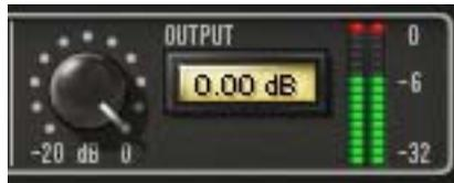
Output controls the signal level that is output from the plug-in. The available range is -20 dB to 0 dB.
