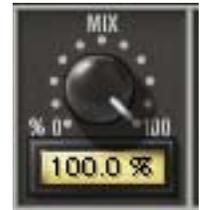
Note that at 0% the signal is still being processed by the band splitter in the plug-in. In linear phase mode the splitter is inaudible, but in minimum phase mode you may hear a slight coloration of the signal at 0%.
