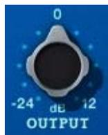
This control provides -24 dB to +12 dB of clean uncolored gain at the output of the plug-in.
