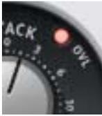
The Overload “LED” illuminates when the signal level at the output of the plug-in reaches  $0$  dBFS. The indicator matches the behavior of the original hardware unit. However, in the software plug-in version, the output can be “overloaded” without causing distortion.
