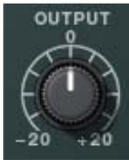
The Output knob controls the signal level that is output from the plug-in. The default value is 0 dB. The available range is  $\pm 20$  dB.
