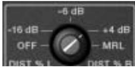
The Manual Cal knob performs two functions: it sets the signal level of the “external” test tone generator for record calibration, and specifies when alignment tapes are to be used for playback calibration.
