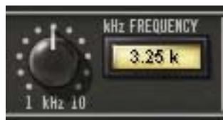
The kHz Frequency parameter defines the cutoff frequency for the enhancement process in Mode A and Mode C. Frequencies above this value are enhanced by the processor. The available range is 1.00 kHz to 10.0 kHz.
