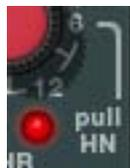
Normally, the limiter and compressor operate with soft knee characteristics. This switch gives the limiter and compressor a hard knee instead.
