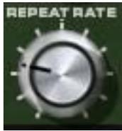
This knob controls the time interval of the echo effect. Rotating the control clockwise will decrease the delay time, and counter-clockwise rotation will increase the delay time.
