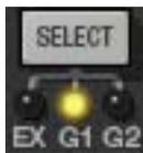
The Select button cycles through the three modes available in the gate/expander module: Expand, Gate 1, and Gate 2.
