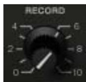
Record adjusts the signal level into the plug-in and the tape circuitry. There are two Record controls, one for the left channel and one for the right. These left/right Record controls can be adjusted individually, or simultaneously when Link mode ([page 26](#)) is active.
