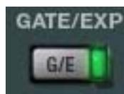
This button activates the gate/expander module. The module is active when the button is gray and the green indicator illuminates.
