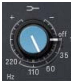
The low band is controlled by dual-concentric knobs, delivering smooth shelving equalization. The inner knob controls the band gain, and the outer ring selects the frequency or band disable.
