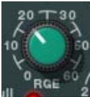
Range (RGE) controls the difference in gain between the gated/expanded and non-gated/expanded signal. Higher values increase the attenuation of signals below the threshold. When set to zero, no gating or expansion occurs. The available range is  $0$  dB to  $-60$  dB.
