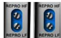
The Repro EQs are used as filters to shape the frequency response of the system in maintaining a flat response and enable compensation for any tape frequency loss or head wear.
