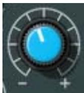
This control determines the amount by which the frequency setting for the HMF band is boosted or attenuated. The available range is  $\pm 20$  dB.
