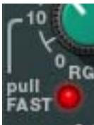
The Fast mode switch defines the gate/expander attack time, which is the duration between the input signal reaching the threshold and processing being applied. Two times are available:  $500$  microseconds (when Fast is off) and  $50$  microseconds (when Fast is active).
