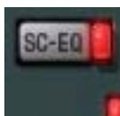
This control enables the UAD Neve 88RS sidechain function. When sidechain is active, signal output from the EQ module is removed from the audio path and is instead routed to control the dynamics module.
