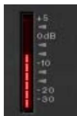
This LED-style meter indicates the level of the signal at the output of the plug-in.
