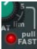
The Fast mode switch defines the attack time (the duration between the input signal reaching the threshold and processing being applied) of the limiter and compressor.
