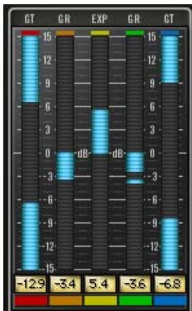
Realtime display of Precision Multiband dynamics processing is shown in the Dynamics Meters. This area also contains the band enable and band solo controls.
