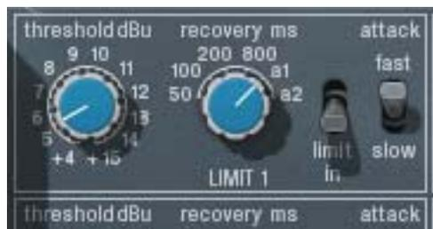
Controls in this section only function when the limiter is enabled with the “limit In” switch (the Power switch must also be on).
