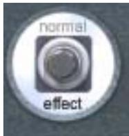
This is an effect bypass switch. Click to enable/disable the chorus or vibrato effect. The effect that will be heard is determined by the Vibrato/Chorus switch.
