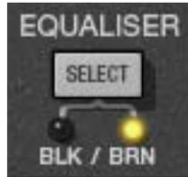
Two different types of SSL EQ are available. The EQ Type button selects between the two types, either Black or Brown. The knob color of the LF band controls changes to reflect the current setting.
