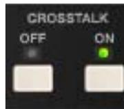
These buttons are global enable/disable controls for the Crosstalk Level (XTALK) parameter. When Crosstalk is ON, the amount of Crosstalk can be adjusted using the Crosstalk Level control.
