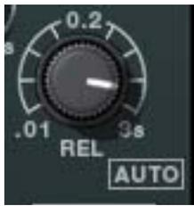
Release sets the amount of time it takes for processing to cease once the input signal drops below the threshold level. The available range is 10 milliseconds to 3 seconds, and automatic.
