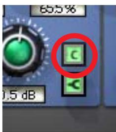
When a band is in shelf mode and its Q is above the minimum value, a resonant peak occurs in the filter response. The Shelf Type button affects where this resonant peak occurs in relation to the shelf frequency.
