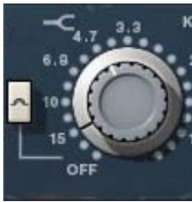
The high band delivers smooth high frequency shelving or peak equalization. The inner knob controls the band gain, and the outer ring selects the frequency or band disable.
