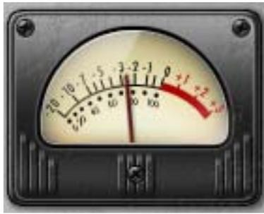
The vintage-style VU Meter represents the plug-in output level. It is active when the Power switch is on, and slowly returns to zero when Power is switched off.
