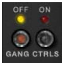
Gang Controls enables global control adjustments of all parameters for all Studer A800 instantiations. This functionality may be accessed from within any active Studer A800 plug-in.
