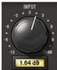
The Input Level knob controls the signal level that is input to the plug-in. Increasing the input will generally result in more processing (depending on the settings of the other parameters).
