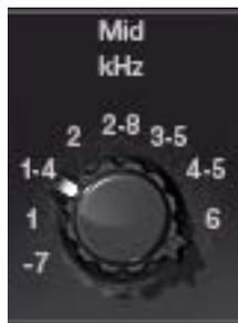
This control determines the frequency of the midrange band. The following frequencies can be specified: 700 Hz, 1 kHz, 1.4 kHz, 2 kHz, 2.8 kHz, 3.5 kHz, 4.5 kHz, and 6 kHz.
