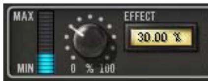
The Effect Knob controls the amount of processing that occurs in the plug-in. The available range is from 0.00 to 100.0%.
