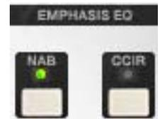
When the value is set to NAB (traditionally the United States standard), the Hum Noise frequency is 60 Hz. When set to CCIR (traditionally the standard in Europe and other regions), the Hum Noise frequency is 50 Hz. See “Noise Enable” on page 34 and “Hum” on page 34 for more information about Hum.
