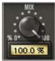
The Mix control determines the balance between the original and the processed signal. The range is from 0% (dry unprocessed signal only) to 100% (wet processed signal only). The default value is 100%.
