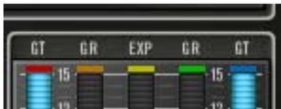
The labels above the Dynamics Meters reflect the mode that each band is in: GR (Gain Reduction) for compression, EXP for expansion, and GT for Gate.
