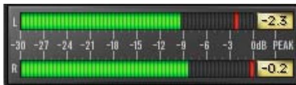
The stereo peak/hold Input and Output Meters display the signal level at the input and output of the plug-in.
