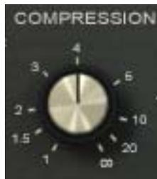
The Compression parameter determines the ratio for the compressor. Less compression occurs at lower values. The available range is continuous, from 1.00:1 to Infinity:1.
