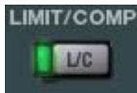
This button activates the limiter/compressor module. The module is active when the button is gray and the green indicator illuminates.
