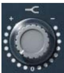
The High Shelf knob offers approximately  $\pm 18$  dB of smooth fixed frequency shelving equalization at 12 kHz.
