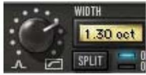
Width controls the bandwidth of the de-essing sidechain when in bandpass mode. Bandpass mode is active when the control is in any position except fully clockwise.
