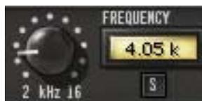
This control defines the center frequency of the de-esser when in bandpass mode, or the cutoff frequency of the de-esser when in highpass mode. For bandpass use, the value is set to the center of the undesirable frequency range that is to be reduced. For highpass use, the value is set below the frequency range that is to be reduced. Used in conjunction with the Width control ([“Width” on page 301](#)), a broad range of de-essing is possible.
