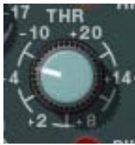
Threshold defines the input level at which limiting or compression begins. Signals that exceed this level are processed. Signals below the threshold are unaffected.
