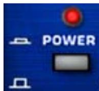
The buttons on MXR Flanger/Doubler are two-state switches. The buttons are ON when they are in the “DOWN” position. When ON/DOWN, they are gray with a darker “shadow.” When OFF/UP, they are white.
