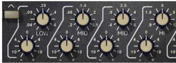
Each of the four EQ bands have similar controls. The band center frequency is controlled the top row of knobs, and the band gain is controlled by the bottom row.
