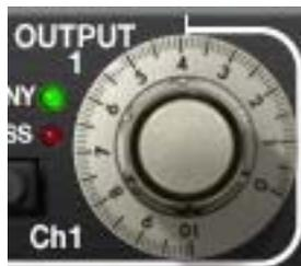
The Output knob controls the signal level that is output from the plug-in.
