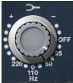
The low frequency band is controlled by dual-concentric knobs, delivering smooth shelving equalization.
