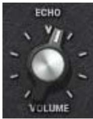
This knob determines the wet/dry mix of the delayed signal. In the minimum position, the “dry” signal is colored by the circuitry of the modeled emulation. Rotate the control clockwise for louder echo. Reducing the control to its minimum value will mute the delay.
