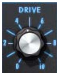
Drive controls the amount of saturation gain before the filter. Drive is where much of the sonic “juice” in the UAD Moog Filter originates. Drive can change the signal from clean to slightly overdriven to extremely distorted, particularly when used in conjunction with the Boost switch (see “Boost” on page 208).
