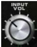
This control determines the signal level that is input to the plug-in. Unity gain is at the 12 o'clock position.
