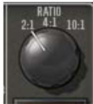
Ratio determines the amount of gain reduction for the compressor. For example, a 2:1 ratio reduces the signal above the threshold by half, with an input signal of 20 dB being reduced to 10 dB.
