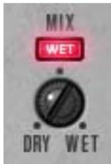
The Mix control determines the balance between the original and the processed signal. The range is from Dry (0%, unprocessed) to Wet (100%, processed signal only).
