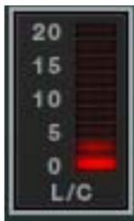
This meter displays the amount of gain attenuation occurring in the limiter/compressor module.
