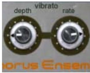
These two knobs control rate and depth of the vibrato effect when CE-1 is in vibrato mode.
