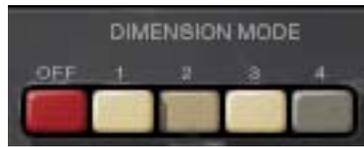
The Dimension Mode determines the effect intensity. Four different modes are available. Mode 1 is the most subtle effect, and Mode 4 is maximum intensity.
