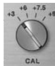
The record, repro, and sync gain trims found on the A800 channel cards are not present on the plug-in. Instead (when "Auto Cal" on [page 433](#) is enabled), these controls are amalgamated into this single Cal Level gain control.
