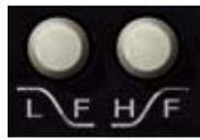
The HF and LF bands are normally in bell mode. When the Bell/Shelf button is engaged for the band (in the darker “down” position), the band is switched to shelving mode.
