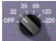
The High Pass filter allows the channel’s higher frequencies to pass while attenuating lower frequencies. The slope of the High Pass filter is 18 dB/octave.
