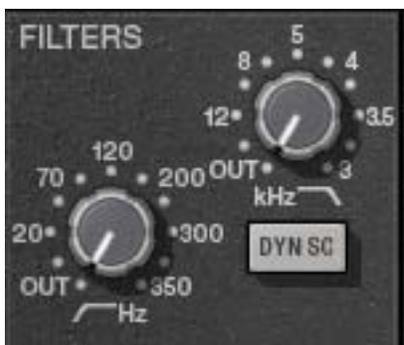
In addition to the four-band EQ, UAD SSL E Channel Strip offers individual high and low pass filters.
