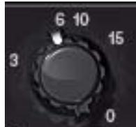
The Bass Gain knob determines the amount of low band gain to be applied when the Bass knob is in one of the frequency positions. Up to +15 dB of boost is available.
