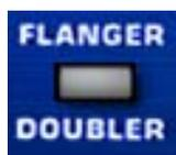
This button switches between Flanger and Doubler modes. It defines the range of signal delay available for the mode. The function of all the other controls is the same in both modes.
