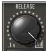
Release sets the amount of time it takes for compression to cease once the input signal drops below the threshold level.
