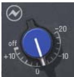
The Input Gain control sets the level at the input of the plug-in, and doubles as a plug-in bypass control. The range is from -20 dB to +10 dB, and off.
