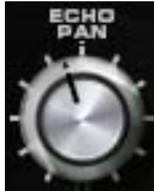
Echo Pan determines the placement of the echo signal in the stereo panorama when the plug-in is used in mono-in/stereo-out and stereo-in/stereo-out configurations. When the RE-201 is used in a mono-in/mono-out configuration, this control is disabled.
