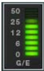
This meter displays the amount of gain attenuation (downward expansion) occurring in the gate/expander module.
