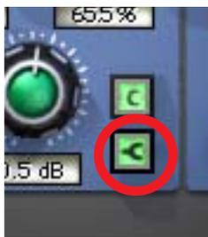
Each band can be switched from parametric mode to shelf mode by clicking the shelf enable button. The button is off by default. To enable shelving on any band, click the shelf button.
