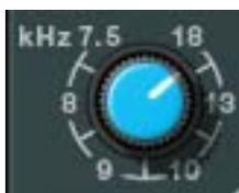
This knob determines the cutoff frequency for the cut filter. The available range is 7.5 kHz to 18 kHz for the high cut filter (lighter blue control), and 31.5 Hz to 315 Hz for the low cut filter (darker blue control).
