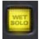
Wet Solo defaults to On, which is optimal when using the EMT 250 in the “classic” reverb configuration (placed on an effect group/buss that is configured for use with channel sends). When the EMT 250 is used on a channel insert, this control should be deactivated.
