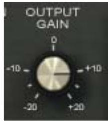
Output Gain controls the signal level that is output from the plug-in. The available range is  $\pm 20$  dB.
