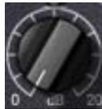
This control determines the amount of EQ gain to be applied to the band. The range is from zero gain (flat) at the fully counter-clockwise position, to the maximum value at the fully clockwise position. Whether the gain is applied as a boost or cut is defined by the Boost/Cut/Out switch (page 192).
