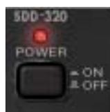
This switch determines whether the plug-in is active. This is useful for comparing the processed settings to the original signal, or to bypass the plug-in to reduce the UAD DSP load (load is not reduced if *UAD-2 DSP LoadLock* is enabled). Click the pushbutton switch to change the Power state.
