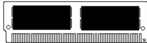
In this example, there are a total of 2 chips, each providing 8 Megabytes of memory.  $8 \times 2 = 16$
