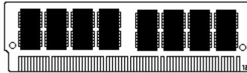
In this example, there are a total of 8 chips, each providing 2 Megabytes of memory.  $8 \times 2 = 16$
