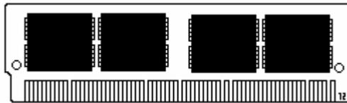
In this example, there are a total of 4 chips, each providing 4 Megabytes of memory.  $4 \times 4 = 16$
