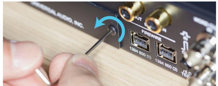
Remove both cover plate screws with the hex wrench.
