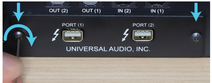
Secure card with the two saved hex screws.
