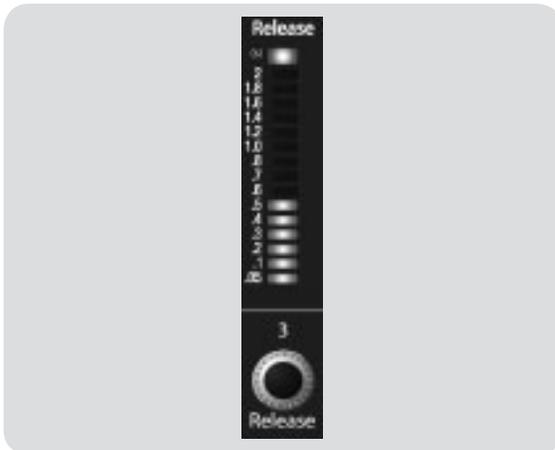
**Sets and Displays the Rate the Gate Closes on the Selected Channel.**
