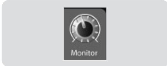
This knob adjusts the overall level of the control-room monitor outputs.
