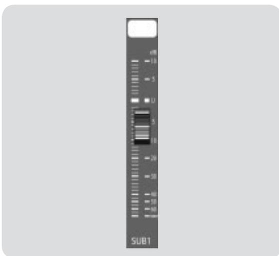
The fader controls the overall volume of the signal on its subgroup output.
