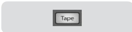
The Tape monitor button routes the signal from the tape inputs (tape returns) to the monitor bus. The level for this input is controlled by the knob in the 2 Track In section.
