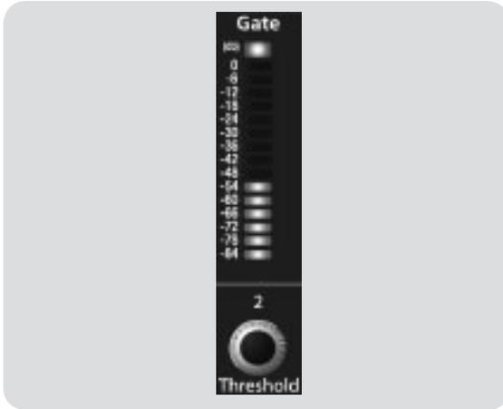
**Sets and Displays the Threshold of the Gate for the Selected Channel.**
