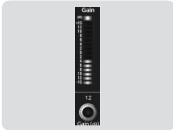
**Sets and Displays the Gain Attenuation or Boost at the Center Frequency of the High Band EQ.**
