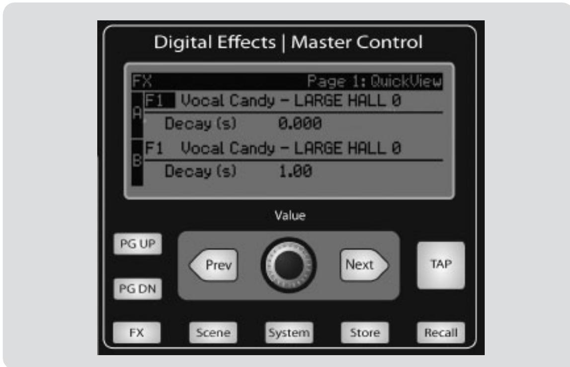
From the Digital Effects | Master Control section, you can select and change the parameters of the two internal effects processors, as well as store and recall every setting on your StudioLive at the touch of a button. Because almost all of the StudioLive's features are controlled from the mixing surface (rather than using menus and submenus), you will mainly use this section to adjust the internal effects processors and to save and recall presets and scenes.
