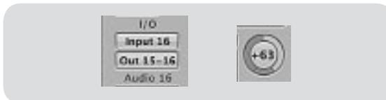
Once you have the routing set up in Logic, record-arm the track and insert the desired plug-in. Press the FireWire Return Input button on your StudioLive. You can now monitor your analog signal with your inserted effect as you record.
