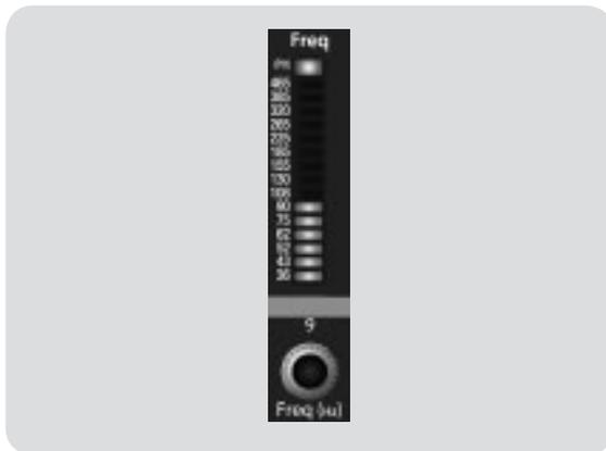
**Sets and Displays the Center Frequency of the Low Band EQ.**
