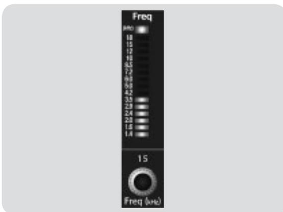
**Sets and Displays the Center Frequency of the High Band EQ.**
