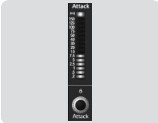
**Sets and Displays the Compressor Attack Setting for the Selected Input Channel or Output Bus.**
