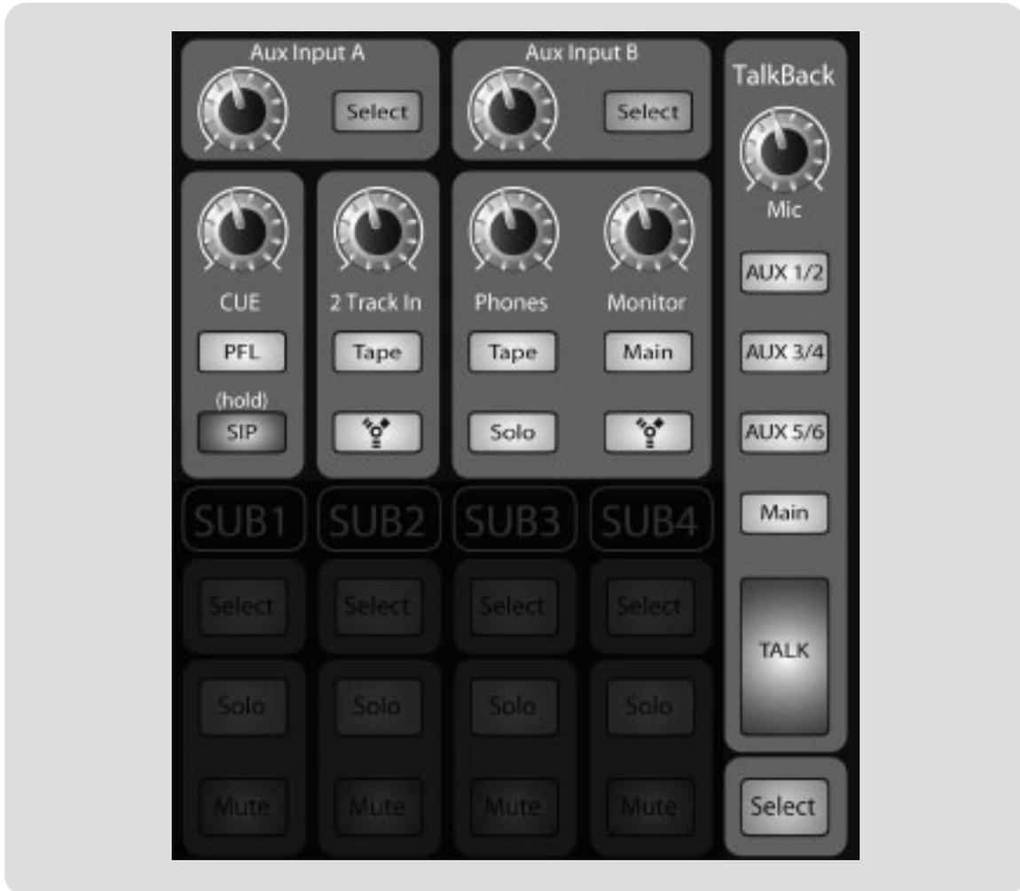
The Master section of the StudioLive controls the monitoring, talkback output, solo bus, and aux and tape inputs.
