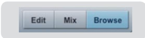
In the lower right corner of the Arrange window are three buttons. The Edit button opens or closes the Audio editor or the MIDI piano-roll editor, depending on what type of track is selected. The Mix button opens and closes the mixer window.
