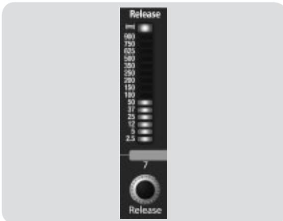
**Sets and Displays the Compressor Release Setting for the Selected Input Channel or Output Bus.**
