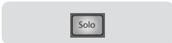
The Solo Bus Monitor button patches any soloed channel, subgroup, or aux send to the Monitor bus. This can be useful in any number of ways; for example:
