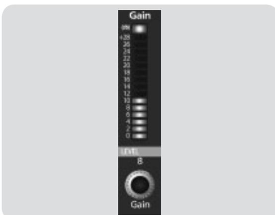
**Sets and Displays the Amount of Makeup Gain for the Compressor on the Selected Input Channel or Output Bus.**
