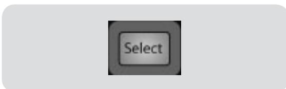
As previously described in section 2.3.1, the Select button routes its channel through the Fat Channel, allowing you to add dynamics processing, EQ, panning, etc.
