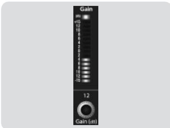
**Sets and Displays the Gain Attenuation or Boost of the Center Frequency for the Low Mid Band.**
