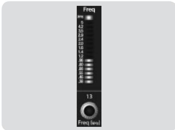
**Sets and Displays the Center Frequency of the High Mid Band EQ.**
