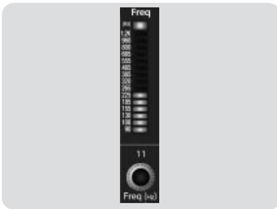
**Sets and Displays the Center Frequency of the Low Mid Band EQ.**
