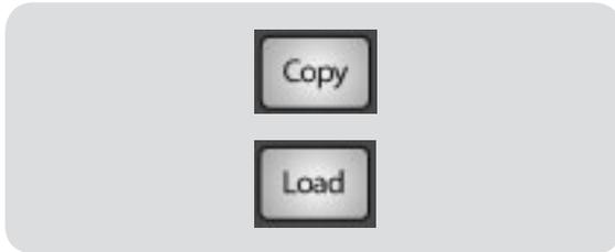
To paste the current channel's Fat Channel setting to another channel or bus, simply press that channel's Select button. It will stop flashing and illuminate. After you have selected every channel to which you want the settings pasted, press the Load button. The StudioLive will return to its normal state, indicating that the Fat Channel settings have been successfully pasted.
