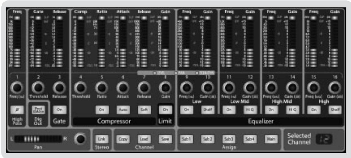
The heart of the StudioLive is the revolutionary Fat Channel. The Fat Channel makes dynamics, routing, and panning for every input and output on the StudioLive available at the touch of a Select button. The 16 multipurpose knobs and meters located in the Fat Channel control nearly every adjustment you will need to make on your StudioLive. From the Fat Channel, you can:
