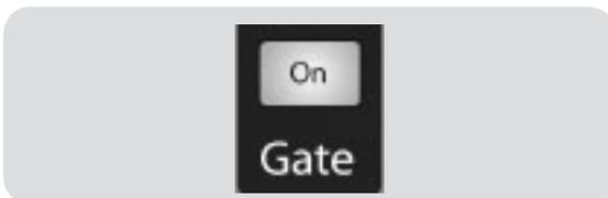
**Turns the Gate On and Off for the Selected Channel.**
