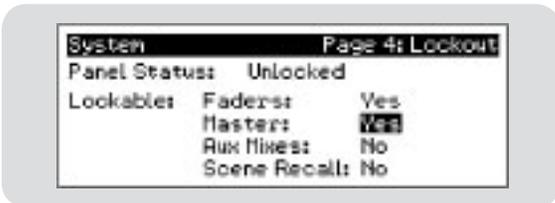
To lock your StudioLive, press the System button in the Digital Effects | Master Control section and navigate to Page 4: Lockout. Your StudioLive cannot be locked unless this page is active. If you have multiple StudioLive mixers connected, you only need to lock the Master unit to lock all the mixers in the chain.
