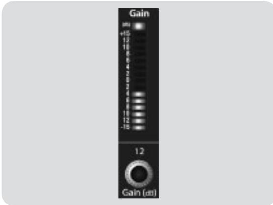
**Sets and Displays the Gain Attenuation or Boost at the Center Frequency.**
