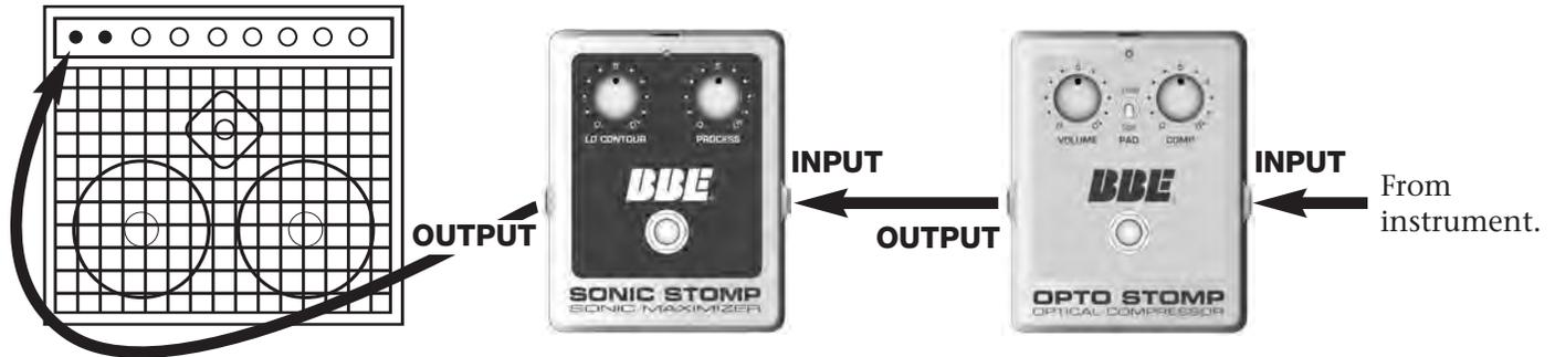
Connect the output of the first pedal to the input of the second pedal. Continue plugging outputs to inputs throughout the chain.
