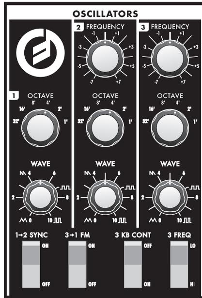
The Oscillators are the main sound source of the Voyager. The oscillators in the Voyager are all analog Voltage Controlled Oscillators, or VCOs. They feature a temperature regulation circuit that provides them with excellent tuning stability. The VCOs can produce a total musical range of 8 ½ octaves! In addition, the frequency of oscillator 3 can be set to sub-audio (<20Hz) vibrations for use as a second LFO.
