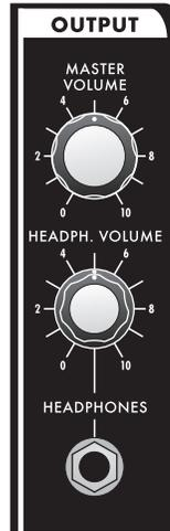
The Voyager has two audio outputs. There is a VCA for each output, which allows for stereo functions such as Panning or the Dual lowpass filtering. The main control for the Volume is the Master Volume Control. The Volume Envelope modulates the output VCAs.
