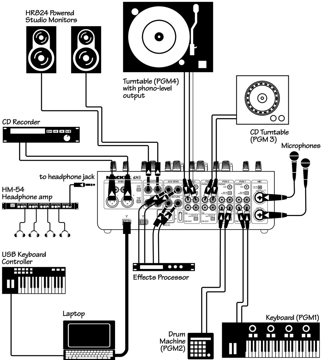
This diagram shows a keyboard, drum machine, turntable and CD turntable, with two microphones. A USB keyboard controller is also attached directly to the computer. The FireWire output from various software, such as Reason™, Ableton Live™, Traktor™, Traktion™, and Logic™ can be sent to the four program channels for mixing. An effects processor is also shown in the aux loop.
