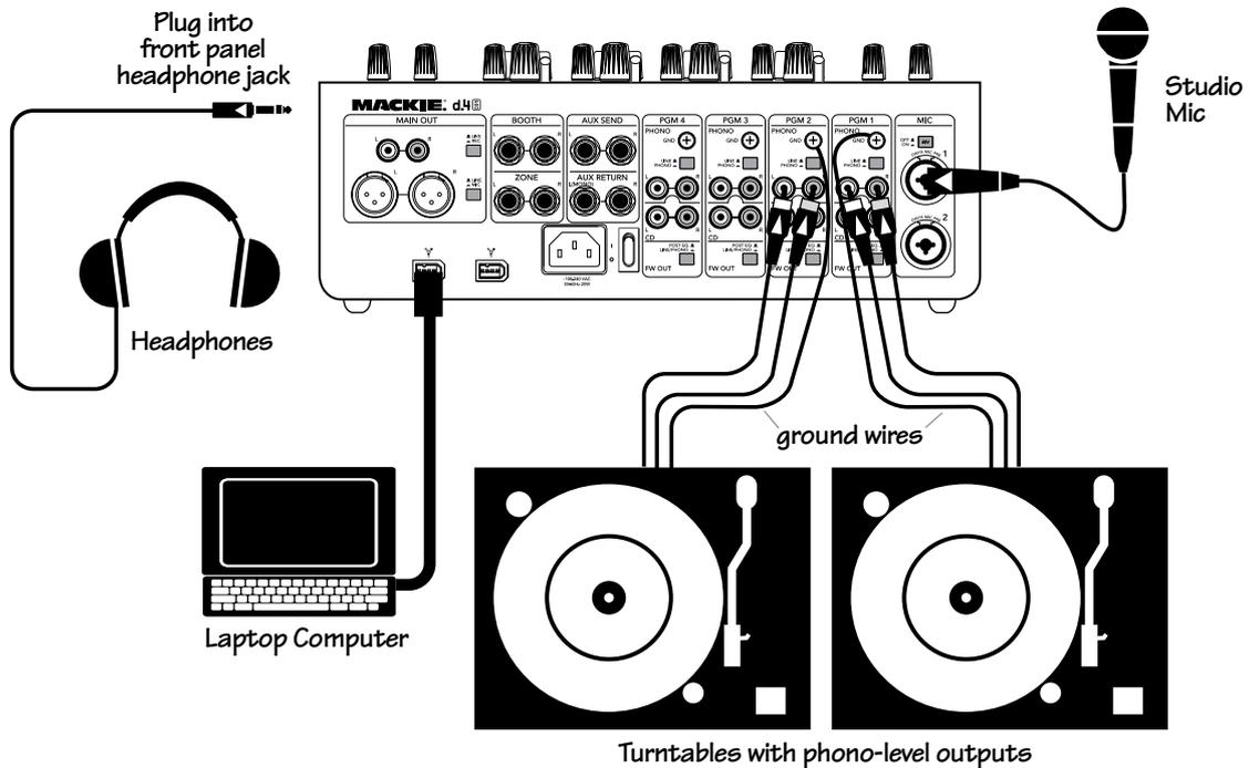
The output from various software, such as Reason™, Live™, Traktion™, and Logic™ can be sent to the program channels for mixing, and the final mix recorded for broadcast/podcasting. This is also a nice setup for recording your record collection for posterity. You could also play timecode vinyl and set up a virtual turntable on the laptop. In this way, you can use the physical turntable to control any musical tracks added to the virtual turntable.
