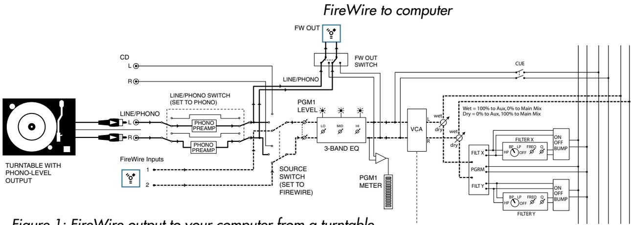
Figure 1: FireWire output to your computer from a turntable
