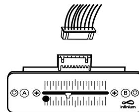
6. Insert the connector into the receptacle on the new crossfader assembly. (It will only fit in one way.)
