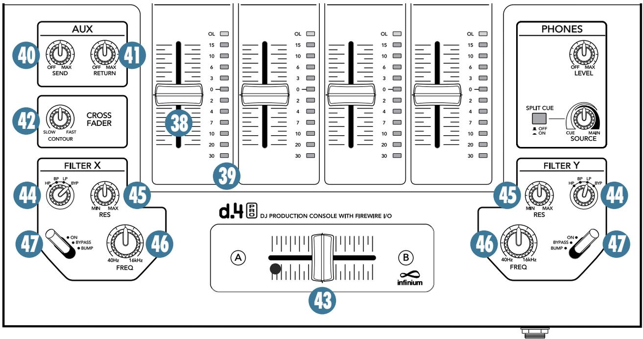
**A CLOSER LOOK** The program faders [38] and the crossfader [43] control the signal levels as follows:
