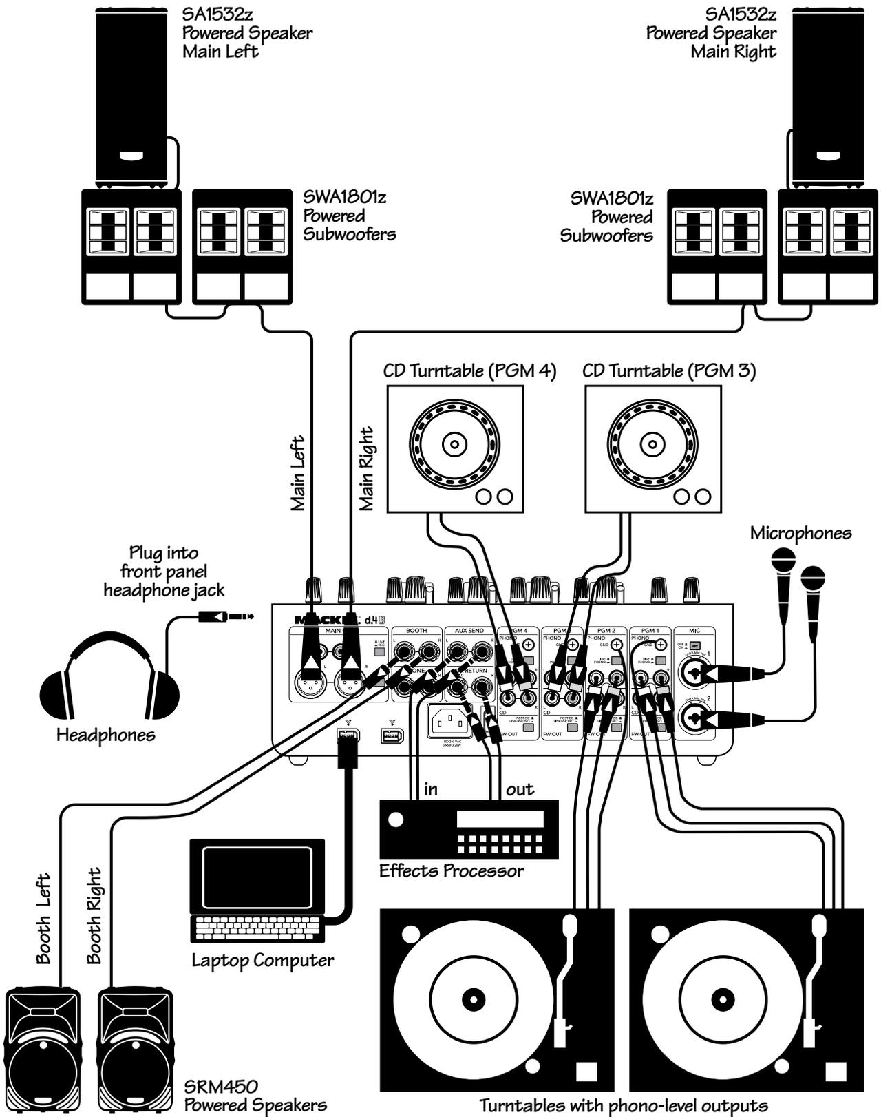
*This diagram shows 4 sources hooked up to 4 channels, with an effects device in the aux loop, and a laptop attached. Separate tracks can be recorded into Traktion, of each stereo program channel and the microphones, and even the effects channel. This gives multitrack recording of all the elements of the performance, for remixing at a later time.*
