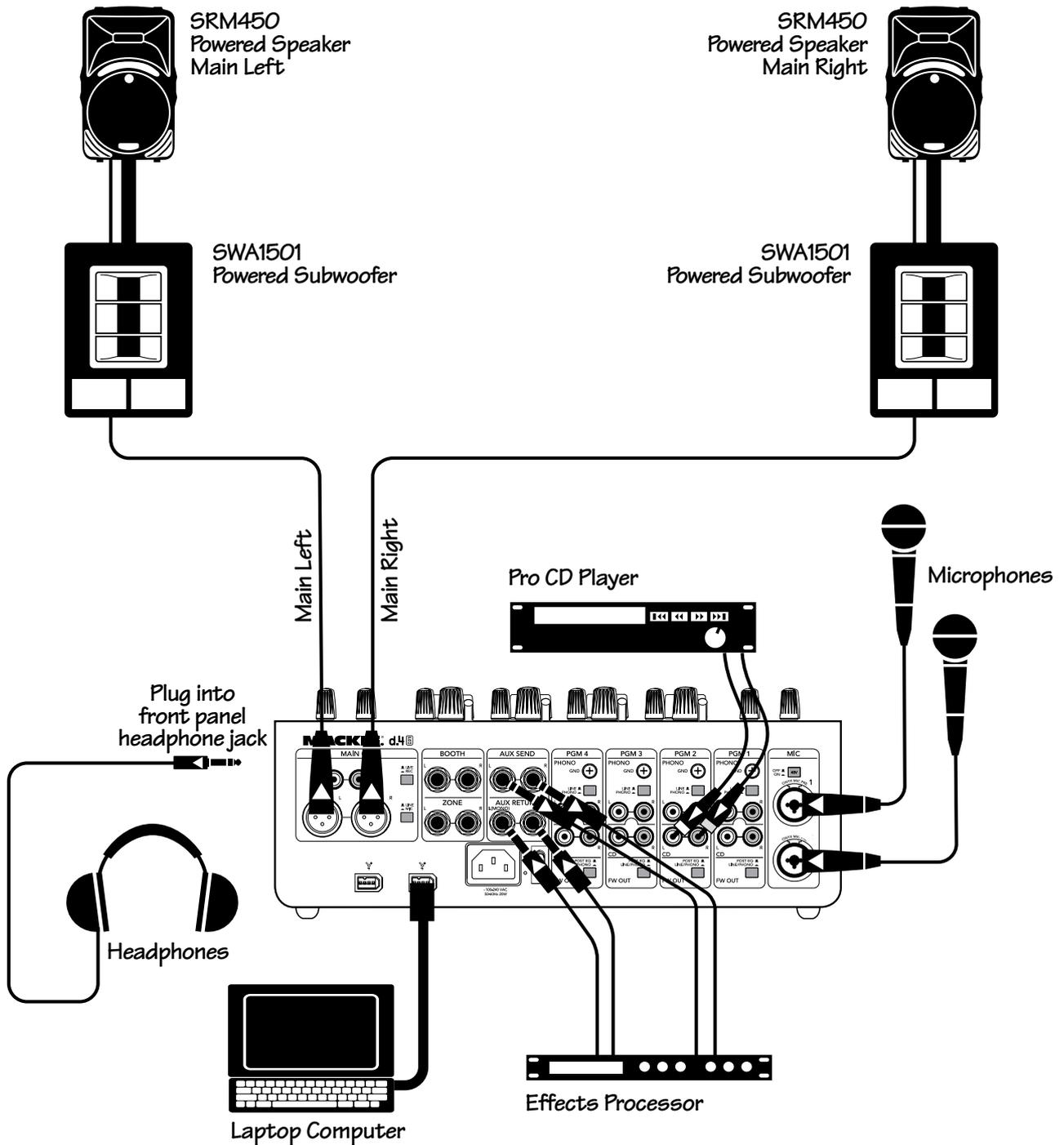
This diagram shows a CD player and microphones connected, with an effects device in the aux loop, and a laptop attached. Various popular DJ software such as Traktor™, PCDJ™, and MixVibes™, can be used with the d.4 Pro via the FireWire connection. The main mix can also be recorded with software such as Traktion.
