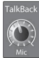
This knob controls the overall volume of the external talkback mic input. The trim for the Talkback mic is located on the back panel next to the input. See Section 3.1 for details.
