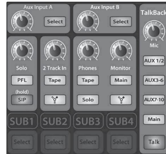
The Master section of the StudioLive controls the monitoring, talkback output, solo bus, and aux and tape inputs.
