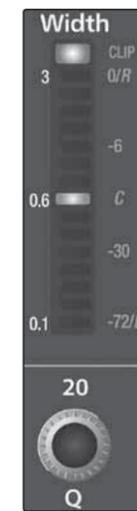
This encoder sets, and the meter displays, the Q for the High-Mid band. The Q is the ratio of the center frequency to the bandwidth. When the center frequency is constant, the bandwidth is inversely proportional to the Q, so as you raise the Q, you narrow the bandwidth.
