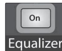
Turns the Equalizer On and Off for the Selected Channel or Output Bus.
