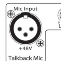
**Talkback Mic Input.** The StudioLive does not have an onboard talkback mic; an external mic must be used. Phantom power is always enabled on this microphone preamp, so either a dynamic or a condenser microphone can be used. This is the same high-quality XMAX preamp that is featured on Channels 1 through 24, and the talkback can be used as an extra input when using the StudioLive as an audio interface. See Section 6.4.2 for details.
