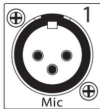
**Microphone Inputs.** Your StudioLive is equipped with 24 PreSonus XMAX microphone preamplifiers for use with all types of microphones. (A 25th XMAX preamp serves the talkback section.) The PreSonus preamplifier has a Class A input buffer, followed by a dual-servo gain stage. This arrangement results in ultra-low noise and wide gain control, allowing you to boost signals without increasing unwanted background noise.
