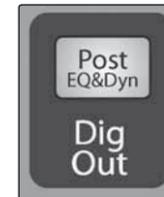
*Note: The Dig Out button does not function when you have a FireWire return selected as an input source. If Dig Out is enabled, any aux, subgroup, and the main bus to which the return is routed will not receive the post-Fat Channel signal. The unprocessed signal will still be routed to these buses, as well as to the FireWire bus, but the Fat Channel processing will not.*
