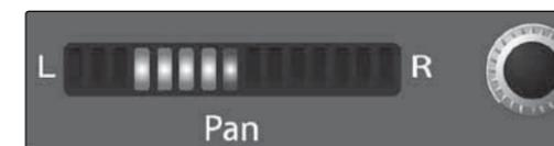
The Pan Control for each Input or Output bus is set on the Fat Channel. The LED display shows the Pan setting, and the encoder to the right of the display controls panning for the selected input or output bus. When two channels are linked as stereo pair, the LED display will automatically change to stereo pan.
