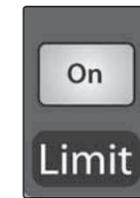
Turns on the Limiter for the Selected Input Channel or Output Bus.
