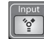
The FireWire Input button routes a playback stream from your audio software to the StudioLive's channel inputs, where it is routed and processed the same way as analog input signals. For example, if you want a particular recorded track to play back on mixer channel 3, simply route that track in your audio software to StudioLive Output 3. This button can also be used to insert a plug-in effect into the mix. For more information on this feature, please review Section 6.4.2.
