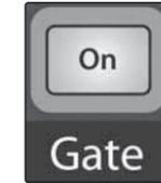
Turns the Gate On and Off for the Selected Channel.
