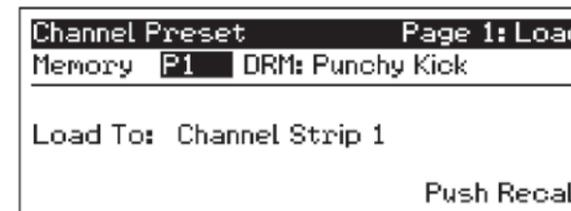
The Channel Preset Load menu always displays the selected channel onto which the preset will be loaded. Use the Value encoder to locate the preset you would like to use. Once you have made your selection, press the Recall button. If at any time you would like to cancel this operation, simply press the Load button again.
