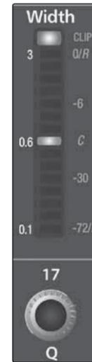
This encoder sets, and the meter displays, the Q for the Low-Mid band.
