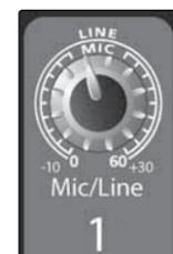
The Trim control adjusts the gain of the channel's analog input.
