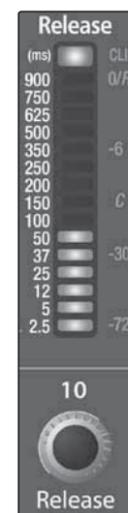
This encoder sets, and the meter displays, the release setting of the compressor for the selected channel or output bus. Release sets the length of time the compressor takes to return the gain reduction back to zero (no gain reduction) after crossing below the compression threshold. Release can be set from 40 to 1,000 milliseconds.
