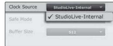
The StudioLive cannot slave to an external clock. However, if you are cascading it with FireStudio-family products that do feature digital inputs, the clock source becomes selectable.
