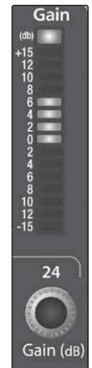
This encoder sets, and the meter displays, the gain cut or boost at the center frequency of the High EQ band. The level of the center frequency can be set between -15 and +15 dB.
