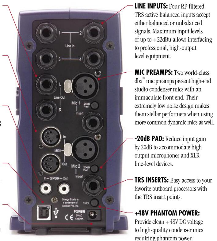
**LINE INPUTS:** Four RF-filtered TRS active-balanced inputs accept either balanced or unbalanced signals. Maximum input levels of up to +22dBu allows interfacing to professional, high-output level equipment.
