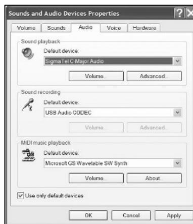
**NOTE:** do NOT choose **USB Audio Codec** as your playback device. This represents your ION Audio USB recording device, and can only be used as a recording input, not a playback output. Also, make sure not to choose **Modem**, or **Microsoft Sound Mapper** as your playback device.
