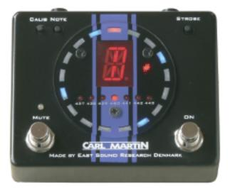
**Calib** – The seven LEDs on the front of the pedal represent seven different calibrations. Pressing the Calib button, allows scrolling through these settings. The calibration settings of the tuner are from 437Hz to 443Hz with the default value at 440Hz. Disconnecting the power source and then reconnecting will reset the calibration to 440 Hz.
