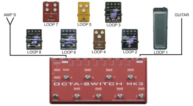
Use a Y-cable in left output with 2 mono and 1 stereo jack, connect Tip & Ring to (+)
