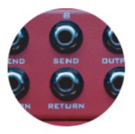
Loop 8 offer a mono send and a stereo return on a stereo jack plug, with left at the jack tip and right at the jack ring. The Octaswitch has stereo outputs, and a stereo return on Loop 8 (this is a stereo jack with tip-left and ring-right). Since stereo effects like choruses are placed at the end of your effects-chain, we would typically insert them in Loop 8.
