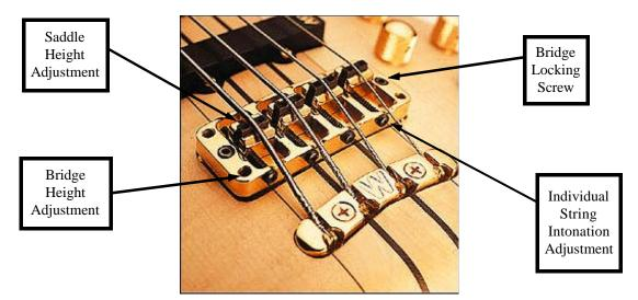
What makes this bridge even more unique is that you can easily change the string spacing of your **Warwick** bass! You can do this by loosening the allen set screw that locks the saddle insert into the saddle. Once you have done that, you can then slide the insert back and forth in the saddle. Be sure to lock the set screw down after you have found the desired string spacing to ensure that your adjustments you have made stay put.
