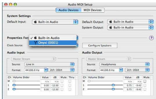
5. Here you can see the settings for the mixer. You can also choose it as your default input or output, as well as designate it to be used for system sound output. There are 12 channels of audio input from the Onyx 1220i, and 2 channels of audio output to the Onyx 1220i.
