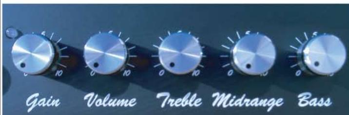
**GAIN** This controls the level of the preamp and acts quite differently than the dirty channel. Turning this control up will add gain, compression, and some slight break up. To get the cleanest signal possible turn the volume to 8 and use the gain knob for loudness.
