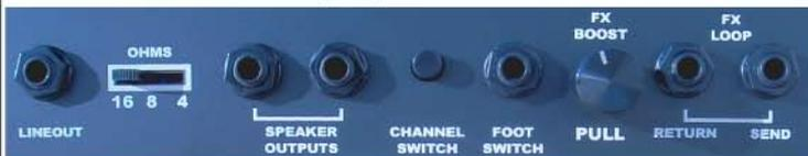
**LINEOUT** This is a line level signal tapped off of the speaker outputs. Under no circumstance should you try to get a signal from this without connecting a speaker load as this will burn the amp up
