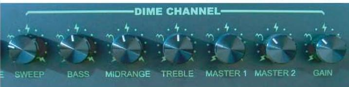
**SWEEP** Shifts the voicing of the EQ section to represent lower frequencies (far counterclockwise) or higher frequencies (far clockwise). This can be used together with the EQ and presence to get a lot of different tones.
