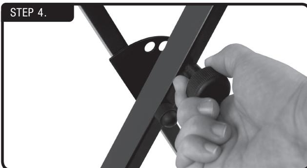
4. To adjust stand height, pull the spring-loaded knob until the pin clears the adjustment plate. Adjust legs until stand is at desired height, then release knob so that the pin snaps into place in one of the holes on the adjustment plate. Do not turn the knob - this can result in the loss of the spring.
