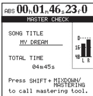
All monitoring is now from the **STEREO** selection only. The master track playback sound is not affected by fader movements or other mixer operations, including new assignments.
