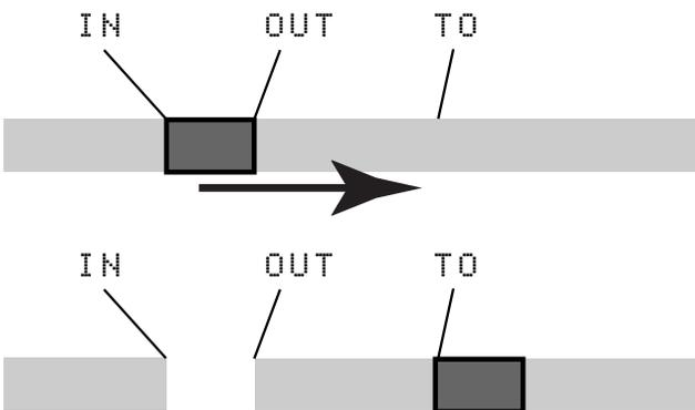
After the operation, the selected section of the source between the IN and OUT points is replaced by silence.
