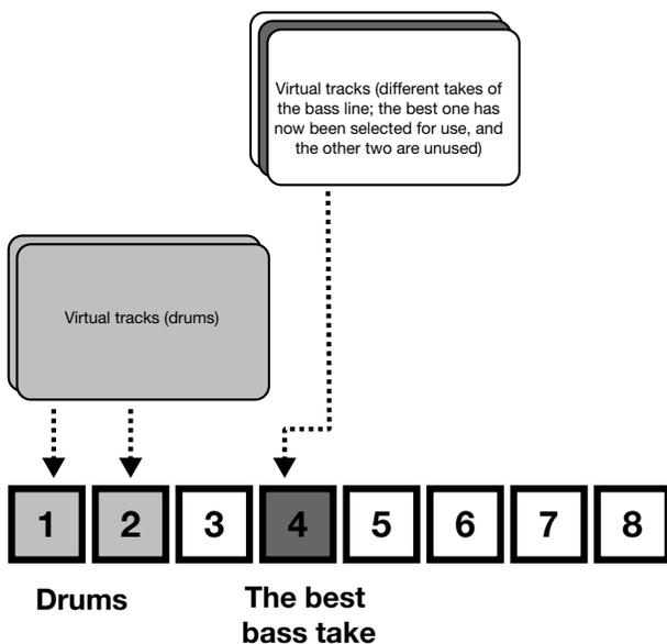
Alternatively, if you want to assemble a track for the whole song, you could assign the three different takes of the part to three different active tracks and use the track editing functions to copy and paste the good parts of each track to make a perfect whole. Then use the two non-perfect tracks with other virtual tracks for new parts.
