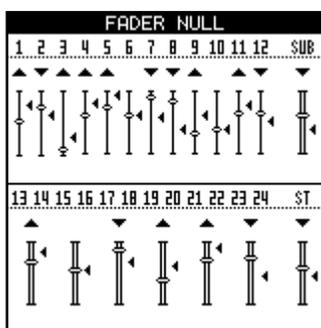
This screen shows the current physical fader positions. The ◀ symbols next to the fader icons show internal fader positions.
