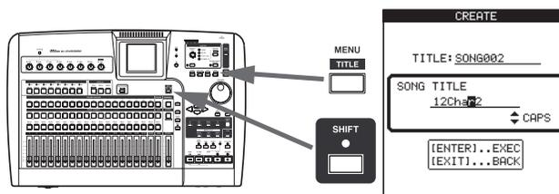
Use the left and right cursor keys to move around inside the title, and the dial to select a character at the cursor position. Use the **INSERT** and **DELETE** keys to insert and delete characters at the cursor position.
