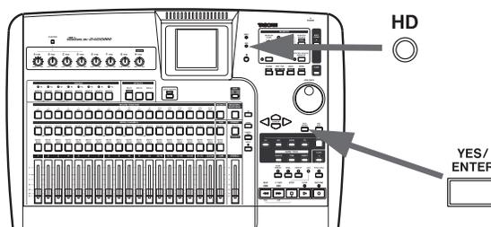
When all data is written to the hard disk, the **SHUT DOWN** indicator flashes red. The display shows `SHUT DOWN COMPLETE`.
