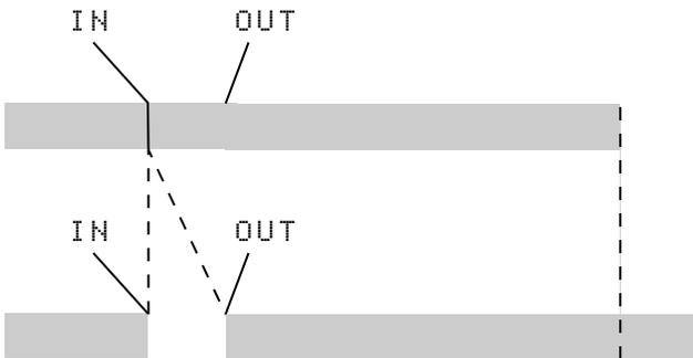
The source and destination are the same, and after the operation, the track is split at the IN point, with the material which followed the IN point now moved to follow the OUT point. The result is therefore longer than the original.
