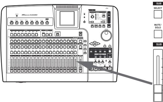
The 2488neo sub mixer facility allows you to add up to eight more inputs (usually on mixdown) to the twenty-four tracks already recorded. These could be inputs from a multi-timbral MIDI device, synchronized using MIDI clock information from the 2488neo driving a sequencer. The eight inputs from **A** through **H** are pressed into service here and they feed a bus that can be routed to the stereo bus (or to the recorder in bounce mix—see “Making a bounce mix” on page 58).
