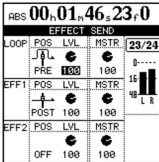
For each effect send, there is a soft switch at the left side of the screen. Use the dial to set this switch either OFF or POST (post-fader) or PRE (pre-fader).
