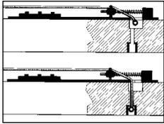
Intonation adjustments can be made by adjusting the intonation screws (A) at the rear of the bridge clockwise to move the saddle back, and counter clockwise to move the saddle forward.
