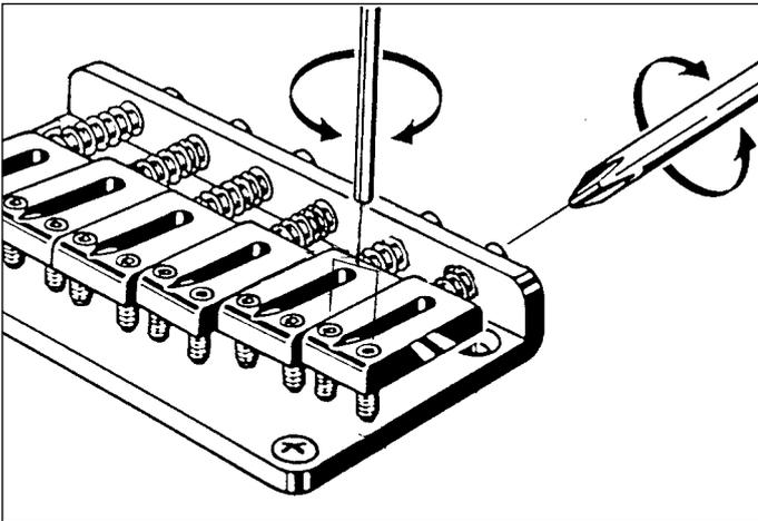
To change strings, thread the new strings through the string grommets located on the back of the guitar and bring them up and over the saddle. The intonation can be adjusted by adjusting the saddle forward or backward using a Phillips (+) head screwdriver on the intonation adjustment screw at the rear of the bridge. String height is controlled by raising or lowering the small Allen screws using a wrench on either side of the saddle.
