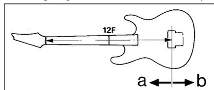
headstock (b) to increase the string length intonation adjustments.
