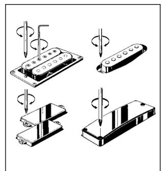
\*Instruments that have adjustable pole pieces can be adjusted to balance the output of each string.
