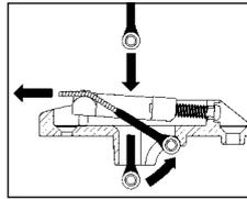
Intonation adjustments can be made by adjusting the intonation screws (A) at the rear of the bridge clockwise to move the saddle back, and counter clockwise to move the saddle forward.
