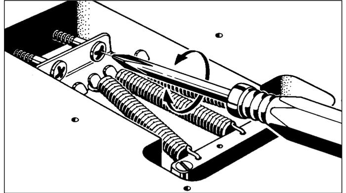
The tremolo springs adjust the tremolo angle by tightening or loosening the tremolo tension. To adjust tremolo angle, locate the adjustment screws in the rear tremolo cavity. The tremolo system when in tune should sit parallel to the surface of the guitar as follows.
