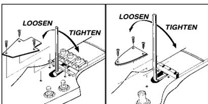
Ibanez steel string models are equipped with adjustable truss rods. The purpose of a truss rod is to adjust the neck to counteract string tension. There are many reasons for truss rod adjustments. One of the most frequent reasons is changing string
