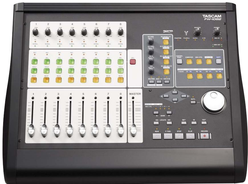
Four microphone inputs, each with phantom power for condenser mics, record to multiple tracks for later overdubbing or mixdown. The first two inputs have analog insert points, so you can insert a compressor to keep from distorting. Up to eight line level signals can be recorded or mixed simultaneously – such as synthesizers or multieffects processors. A S/PDIF connection allows you to connect digital sources for pristine audio quality.
