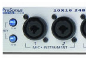
**NOTE: Active instruments are those that have an internal preamp or a line level output. Active instruments should be plugged into a line input rather than into an instrument input. In other words, don't plug an active instrument into the combo jacks on channels 1 or 2.**
