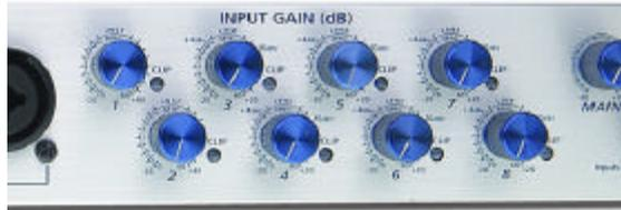
**Clip Indicator.** The clip indicator will light up if your input signal from the XLR (Mic) or ¼" (line) reaches +18dBu (0dBfs). At this level, your mic preamp/line trim signal may not exhibit signs of clipping such as distortion. However, this level would cause the A/D (analog to digital) converters to clip. Therefore it is highly recommended that you do not allow your converters to clip (the clip indicators to light up) as the sound quality would not be desirable.
