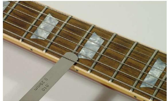
Use common sense and don't force truss rod adjustments! If you feel abnormal resistance to movement, or if the neck is significantly out of spec, it would be prudent to leave further work to a qualified technician.
