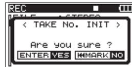
4. Press the **ENTER/MARK** button again to reset the number that follows the characters to "0000". Press the **MARK** button on the top of the unit to return to item selection on the REC page.
