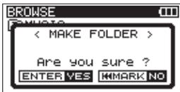
Press the **ENTER/MARK** button to create a new folder. New recorded takes are saved in this folder.
