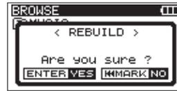
Rebuilding refreshes the take information inside the selected folder, and recognizes files that are not contained in takes as independent takes, making their playback possible. Use this function after you have copied files to the SD card from a computer, for example.
