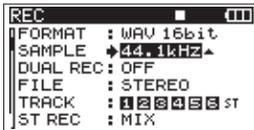
3. Use the **DATA** wheel to select one of the following options: 44.1kHz (default value), 48kHz, 96kHz, or 192kHz.
