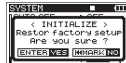
Press the **ENTER/MARK** button to initialize the unit. Press the **STOP** button to cancel initialization.
