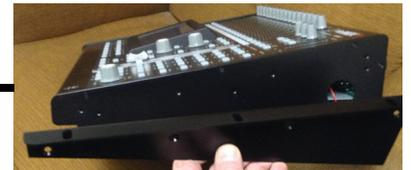
**Step 6:** Fasten the rack ear to the chassis using the four screws as shown.
