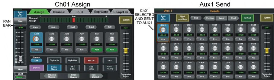
Figure 4.7a: No Linking, Ch01 sent to Aux1 only
