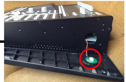
**Step 3:** Gently disconnect the wire assembly header that powers the illuminated Ashly logo. Pull apart by holding the white plastic header rather than the pulling on the wires. Observe connector polarity when reconnecting later, and note that the connector is indexed and can only be inserted one way.
