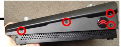
**Step 2:** The plastic sides have an illuminated Ashly logo embedded in the molded plastic. This must be disconnected before the side can be completely removed.
