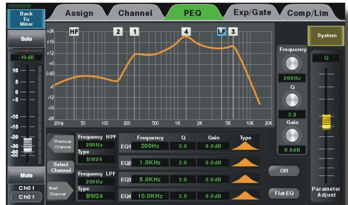
Figure 4.2: PEQ Parametric EQ Screen
