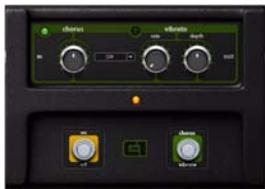
Based on a heavyweight late-70s analog chorus/vibrato pedal, C1 Chorus/Vibrato offers warm, liquid modulation effects. In Chorus mode, the signal is routed through a modulated short delay, which is mixed with the dry signal, creating a washy, doubled sound.
