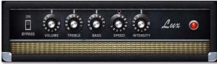
The amp we based the '64 Black Panel Lux Vibrato and Normal models on is regarded by some as the ultimate small club amp. A 60s tube combo with a single 12-inch ceramic-magnet speaker and a pair of 6V6s putting out just over 20 watts, this amp has long been a standard in the studio as well as onstage.
