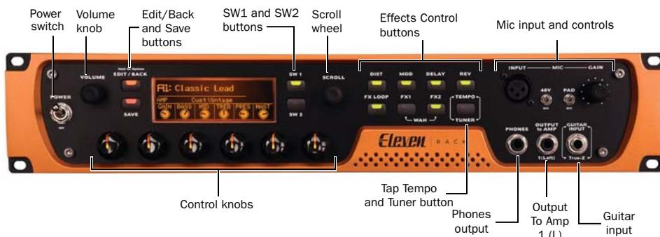
Figure 1. Eleven Rack front panel
