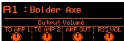
This mode offers fast access to the output settings for the current Rig, using four lit control knobs, labeled TO AMP 1 (Output To Amp 1 volume), TO AMP 2 (Output To Amp 2 volume), AMP OUT (amp output volume), and RIG VOL (Rig output volume).
