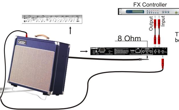
The internal loudspeaker should be plugged into the 8 Ohms socket.
