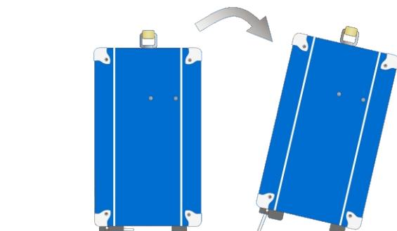
Use this design feature with caution, due to the ease with which the amplifier can be moved between straight and tilted back positions, only use the amplifier on a level, stable surface. DO NOT operate the amplifier on a desk, table, shelf or otherwise unsuitable nonstable platform.
