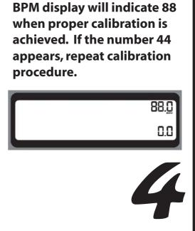
The procedure must be repeated (steps 1 through 4) for the Right Pitch and Wheel calibration.
