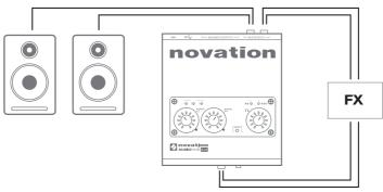
In this setup RCA outputs 1 & 2 are connected to a pair of powered monitor speakers. Outputs 3 & 4 are connected to the input of an external effects processor. The outputs from the effects processor are connected to the RCA inputs on the Audiohub and the Input Monitor switch is pressed in.
