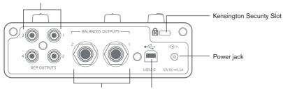
1/4" TRS jack sockets for balanced outputs 1&2 USB socket
