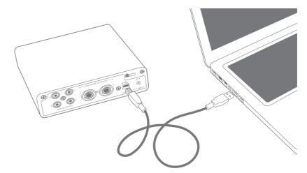
Note: To use Audiohub as a USB hub as well you need to connect the included power supply.
