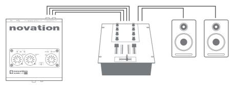
In this setup Audiohub can be used with all four channels connected to a DJ mixer. Audiohub will output two stereo pairs directly from PC or Mac that can then be controlled further on the mixer.
