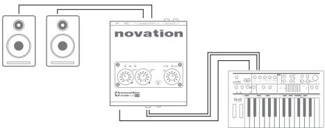
In this setup the two main jack outputs 1 & 2 are connected to a pair of powered monitor speakers, and a device such as a synth is connected to the RCA inputs (an audio cable will be needed as shown above). If the device is USB bus-powered it can be plugged into the Audiohub's USB ports on the front. The input monitor switch is pressed in to mix the device's sound directly with outputs 1 & 2.\*
