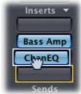
During the drag and drop operation, the potential destination is displayed as an orange rectangle (empty slot) or line (when placing an effect between two Insert slots, see below). Pressing Option during dragging copies the plug-in.
