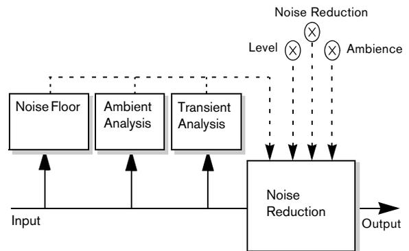
The solid line represents the actual audio signal, while the dotted lines represent control signals
