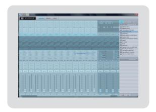
To load a new scene on your StudioLive, select it from the Browser window and drag it over the mixer in either the Overview or the Channel tab. The window will grey out indicating that a new scene is about to be loaded. Please note: only the parameters that have been enabled for recall on the StudioLive will be recalled on the mixer.
