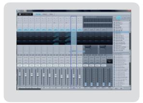
To load every component in a Fat Channel preset (Gate, Compressor, EQ), select it from the Browser window and drag it over any part of the desired channel. If you drag it over any of the component quick views, it will load only that component (i.e. if you drag a preset over the Gate Quick View, only the Gate will be loaded)
