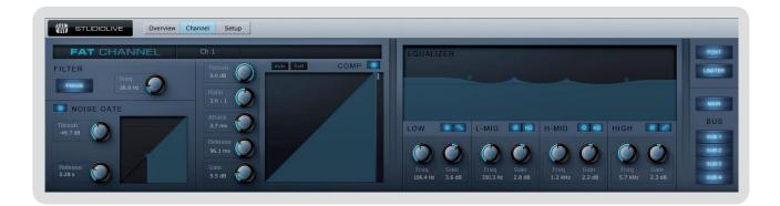
The Channel Tab provides a detailed over view of the Fat Channel parameters for the Selected Channel. The Selected Channel will always be shown above the Gate section. It is important to remember that you have continuous bi-directional control. If you wish to grab a point in the EQ with your mouse, for example, you will be changing the parameters both in VSL and in real-time on your StudioLive.
