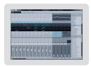
To load a graphic EQ preset, select the preset from the Browser window and drag it over any part of the graphic EQ in the Master section of the Overview tab. Once it is loaded, you can use the sliders in VSL or the encoders on the StudioLive to make adjustments. Note that you must be on the GEQ page in the System menu to have control over the graphic EQ in VSL from the StudioLive.
