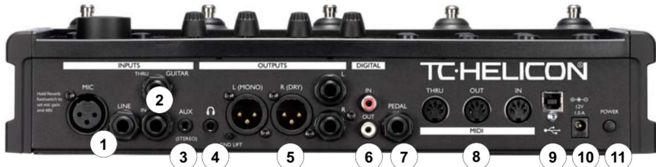
**1. MIC and LINE inputs** - Connect your microphone or line level audio device's output here. Only one should be connected at a time. Hold the REVERB footswitch to set gain when changing back and forth between MIC and LINE ins.
