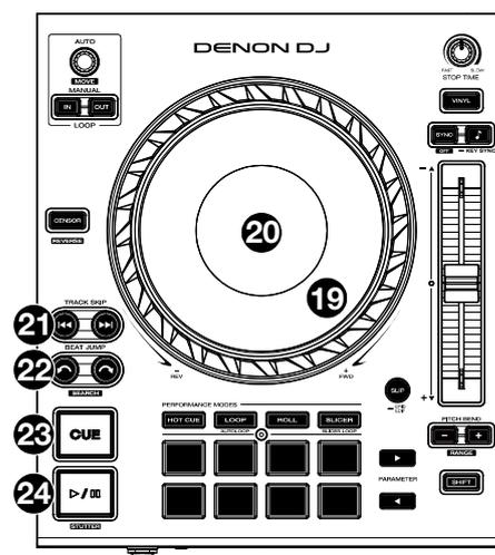
25. **Stop Time:** Controls the rate at which the track slows to a complete stop ("brake time") when you pause it by pressing **Play/Pause**.
