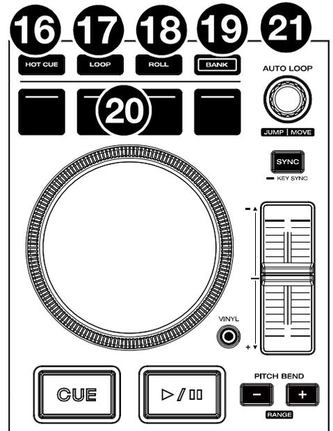
22. **Sync:** Press this button to activate sync. When Key Lock is activated, the track's key will remain the same even if you adjust its speed.
