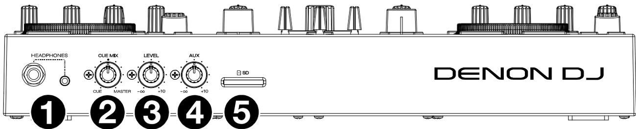
1. **Headphones (1/4", 1/8") (6.35 mm, 3.5 mm):** Connect your 1/4" or 1/8" (6.35 mm or 3.5 mm) headphones to this output for cueing and mix monitoring. The headphone volume is controlled using the **Phones Level** knob.
