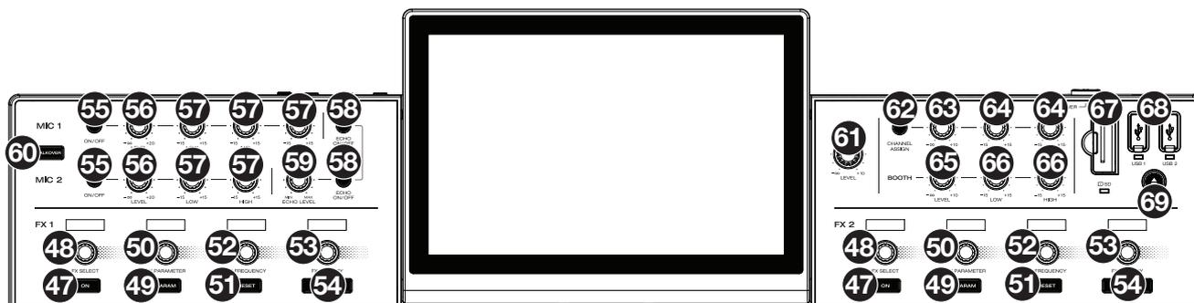
47. **FX On:** Press these buttons to enable or disable FX 1 and FX 2.
