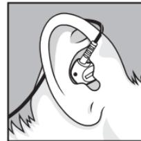
Westone UM monitors come with two sizes of eartips. Use whichever is most comfortable and provides the best seal for you. To remove and replace the eartips, rotate counter-clockwise and pull gently. You may order replacement eartips through our Online Store at [www.westone.com](http://www.westone.com) or by calling our Supply Line at 1-800-582-4771.
