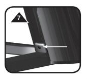
7. To accommodate larger, heavier keyboard and / or lower playing styles, remove angle adapter and re-adjust stabilizer. This changes column angle and shifts center of gravity.
