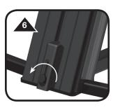
**6.** Loosen thumbscrew and slide stabilizer to touch the floor. Re-tighten the thumbscrew.
