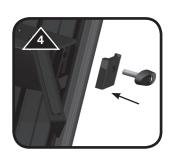
Position clamp on column face and install bracket and T-screw. (Angular edge rides in column slot.)
