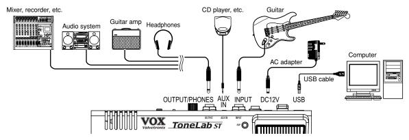
Set the AMP/LINE switch appropriately for the type of device you'll be connecting to the OUTPUT/PHONES jack. Set the AMP/LINE switch as follows.
