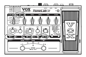
2. Press the AMP bank select switch to select a bank, and use the AMP selector to select an amp model.
