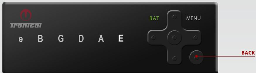
Upon completion of measurement the system switches to the **BLUE** (User) bank automatically indicated by the **BLUE FLASHING LED**.
