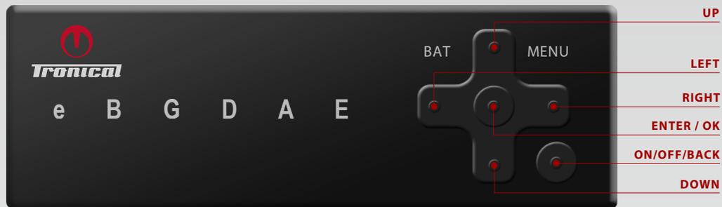
**i** PUSH AND HOLD THE "OFF-BUTTON" TO SWITCH OFF THE SYSTEM.
