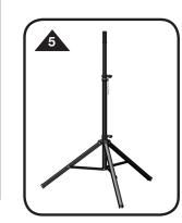
STEP 1 Loosen leg fitting hand knob. STEP 2 Slide leg fitting down to maximum diameter of leg spread (leg braces should be
