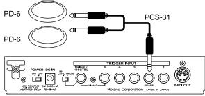
In this case, the white plug tip is connected to TRIG 2 (head), and the red plug tip is connected to TRIG 2 (rim).
