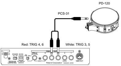
In this case, the white plug tip is connected to TRIG 3 or 5 (head), and the red plug tip is connected to TRIG 4 or 6 (rim).
