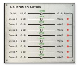
In order to be properly calibrated, the VU meters need to display 0dB with a 1kHz sine wave is played at -18dBFS, with an -18dB Calibration Level.
