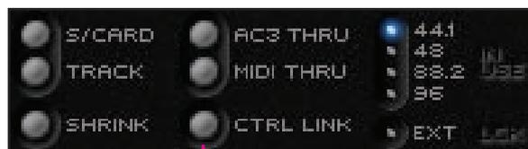
**CTRL LINK switch – engage to link the Level controls for all Analogue Outputs (in the centre of the window)**
