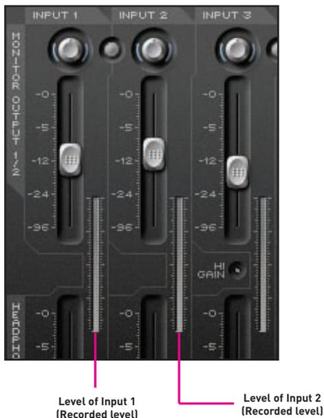
If recording a stereo signal then make sure that the Gain dials for both Inputs on the front of the hardware are set to the same level, observing the Input meters in the SaffireControl LE software, shown above.
