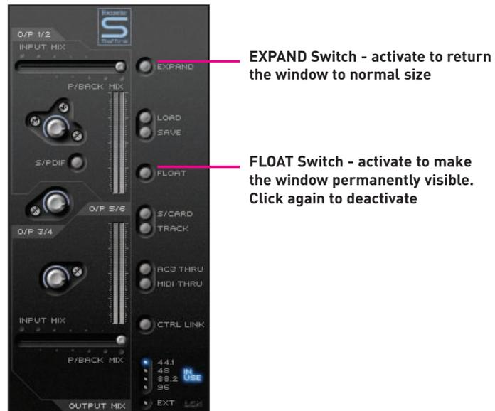
Furthermore, the FLOAT switch activates a mode where the SaffireControl LE window is always visible so that, even when editing in your sequencer, the interface settings can always be seen. SaffireControl LE will FLOAT in normal or 'shrunken' modes. Whilst shrunken, an EXPAND switch is available for returning the window to normal size as shown above.
