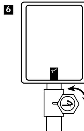
Loosen collar handknob and raise equipment to the desired height. **Do not extend the center pole more than 36" (91.4 cm) above the locking collar support.** Re-tighten handknob and check the stability of the unit at the desired height setting.
