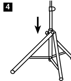
Turn tripod upright and slide leg fitting to adjust the width of the leg spread until the center pole is approximately 1/4" (64 mm) from the floor. This will ensure the Passport tripod speaker stand is at its maximum footprint (Using a smaller footprint will adversely affect the stability of the unit). Tighten the handknob.
