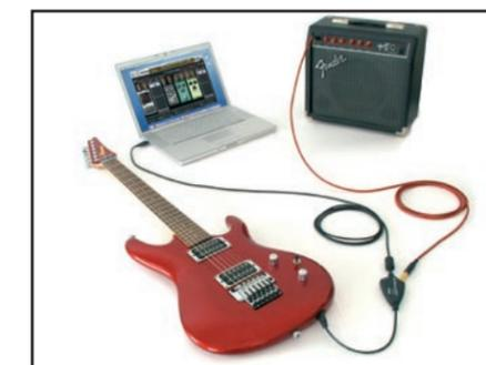
• You can use the StealthPlug as any standard audio interface integrated with your preferred sequencer for recording and processing with the included plug-in
