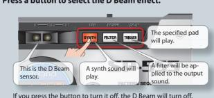
Position your hand above the D Beam sensor, and slowly move it up and down. The sensitivity of the D Beam controller will change depending on the amount of light in the vicinity of the unit. If it does not function as
