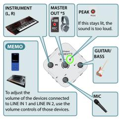
\* 5: The [MASTER OUT] knob adjusts the overall volume that is recorded.
