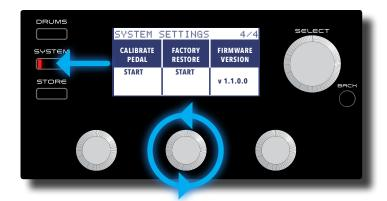
**WARNING!** Performing the factory restore procedure will restore all user presets back to their factory default state. Any changes you have made and stored to user presets will be lost! Once performed, this procedure is irreversible.
