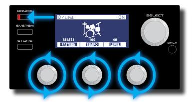
**NOTE:** The Looper and Drum Machine cannot be used at the same time. If you have recorded a loop using the Looper, you must first clear the loop before turning on the Drum Machine. To clear the loop, enter the Performance state and press **FOOTSWITCH 3** two times quickly to stop loop playback. With playback stopped, press and hold **FOOTSWITCH 3** for 2 seconds to clear the recorded loop.
