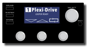
Stomp Mode, and Bank Mode. For more information on these Footswitch Modes, see Footswitch Modes on page 41. In the Performance state you can also control the Preset Level and Master Level parameters by turning the EDIT I and EDIT 3 knobs. See Preset Level & Master Level on page 25 for more information on these output level parameters.
