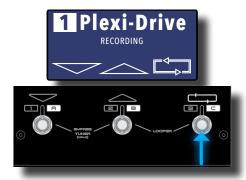
**NOTE:** The Looper and Drum Machine cannot be used at the same time. If the Drum Machine is turned on, you must first turn it off before you can use the Looper. To turn the Drum Machine off, press the **DRUMS** button twice.
