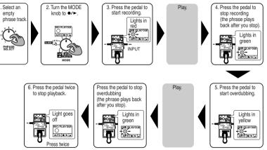
\* For instructions on how to stop playback or overdubbing, refer to "Technique for Stopping Operation" (p. 6).
