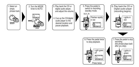
\* For instructions on how to stop playback, refer to "Technique for Stopping Operation" (p. 6).
