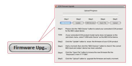
Connect QconPro X to your Mac/PC with the provided USB cable and launch iMap. Click "Firmware Upgrade" to launch the window and follow the steps below carefully to upgrade
