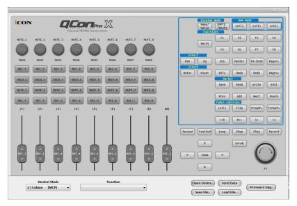
There are controls including faders, knobs, buttons and jog wheel etc. on QconPro X that you could set your own MIDI messages. Four types of message including "Pitch", "Note" & "CC" value you may adjust depended on the control element. Please refer to the below table for different control available setting values.
