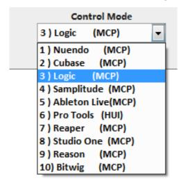
There are two different methods for setting up your QconPro X. In general, it is simpler and faster to set the device to pre-mapped DAW modes with Mackie Control/HUI protocol, depended on which DAW you use. The device has built-in DAW Mackie/HUI protocols as follows:
