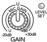
For mono channels (mic input with a mono line input), the gain knob adjusts the input sensitivity of the mic and line inputs.
