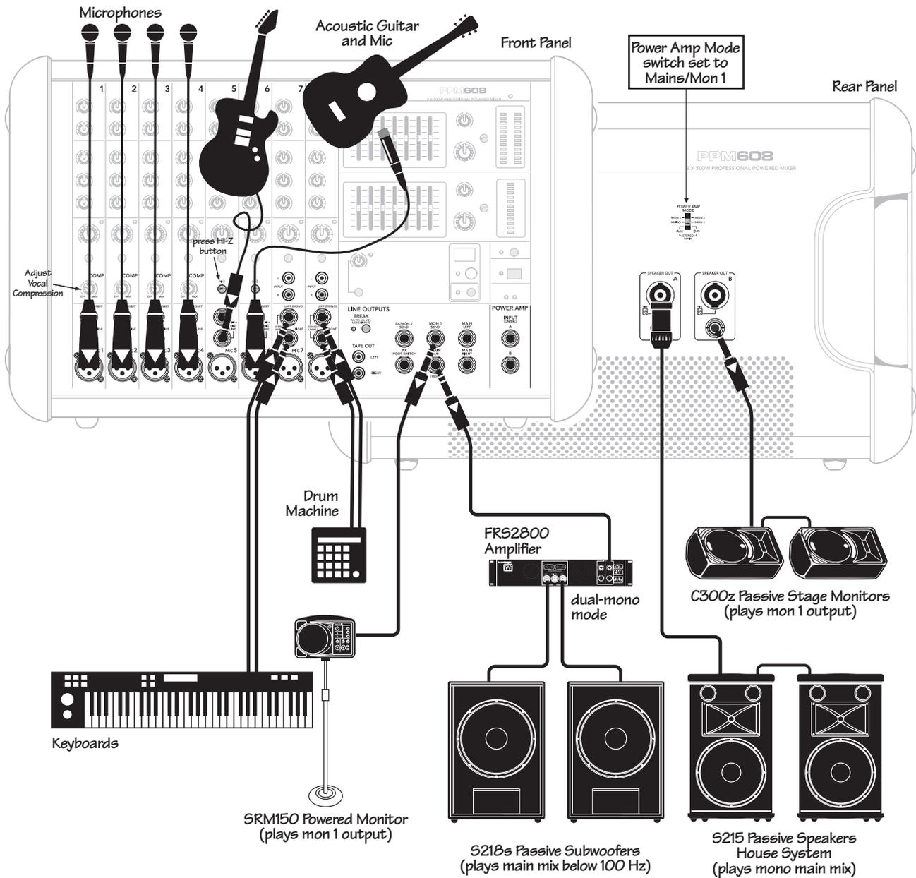
This diagram shows microphones attached to the mic inputs of channels 1 to 4, an electric guitar connected directly to channel 5 (with hi-z switch pressed in), an acoustic guitar microphone connected to channel 6 mic in, a keyboard attached to channel 7's stereo inputs, and a drum machine to channel 8.
