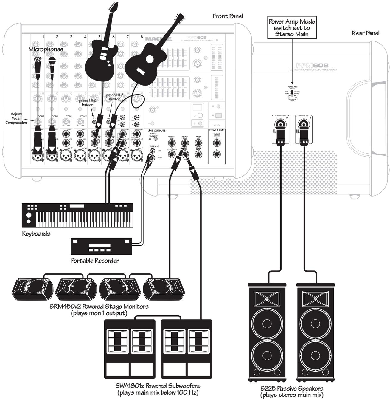
This diagram shows microphones attached to channels 1 and 2, electric guitars connected directly to channels 5 and 6 (with hi-z switch pressed in), and a keyboard attached to channel 7's stereo inputs. A portable recorder is attached to the stereo tape outputs to record the performance.
