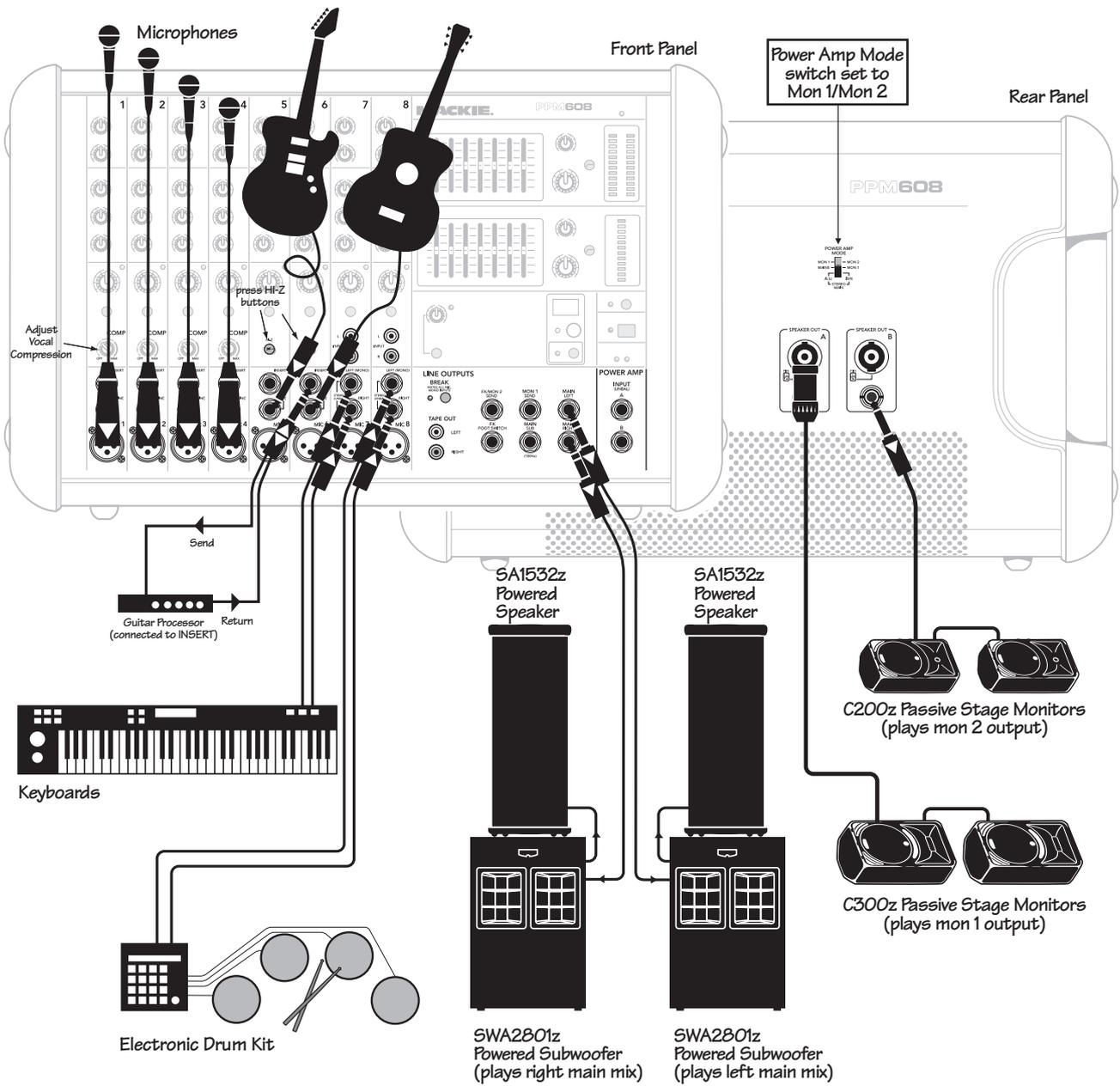
This diagram shows microphones attached to the mic inputs of channels 1 to 4, electric guitars connected directly to ch. 5 and 6 (with hi-z switch pressed in), a guitar processor connected to ch.6 insert, a keyboard attached to channel 7's stereo inputs, and an electronic drum kit attached to channel 8. Add vocal compression as required, by tweaking the compression knobs on channels 1 to 4.
