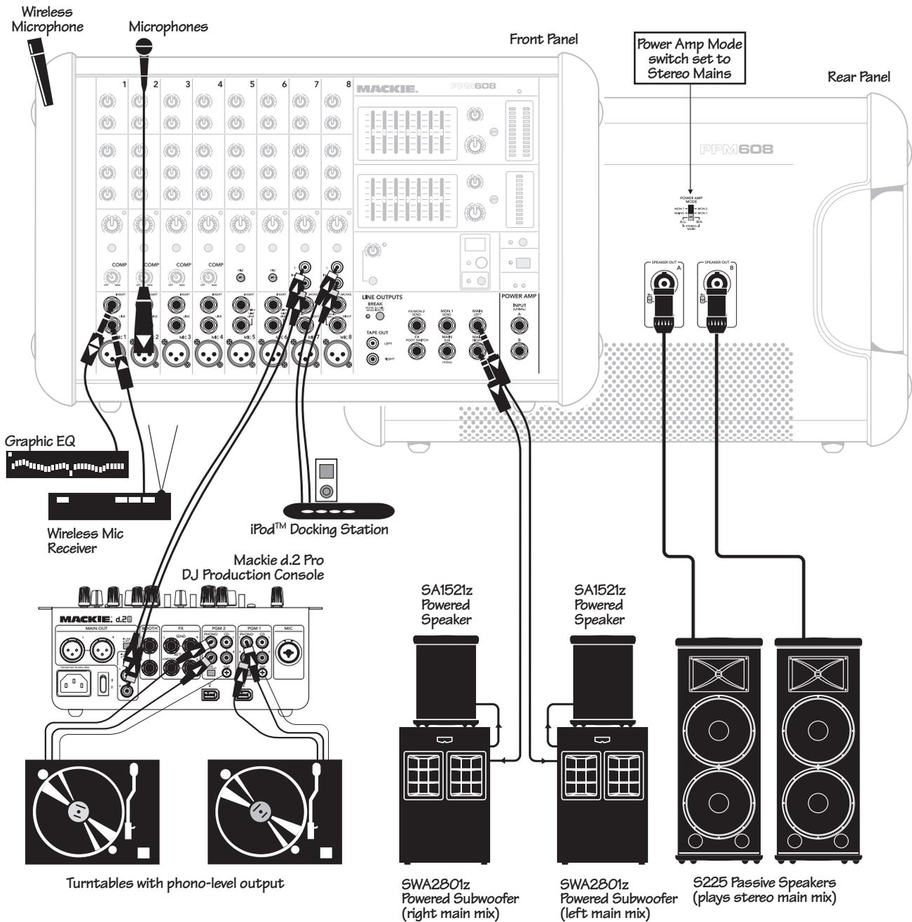
This diagram shows a wireless microphone receiver connected to the channel 1 line input, a graphic EQ connected to channel 1's insert jack (to help control feedback in the wireless mic), a microphone connected to channel 2, and an iPod docking station attached to channel 8's RCA inputs.
