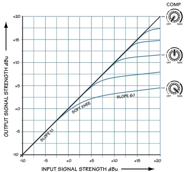
The other blue curves represent in-between positions of the compressor knob, with higher thresholds before compression begins.
